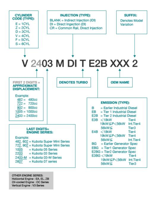
NOTE: The model name above is not printed or stamped anywhere on the engine. It can be found on the Illustrated Parts List (parts catalog).
