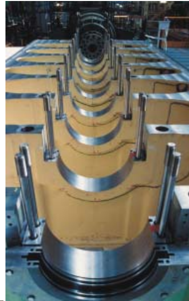
Bedplate of 7RT-flex60C engine.
