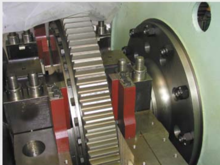
Thrust bearing of 7RT-flex60C engine with the supply unit drive gear on the thrust collar. The flywheel is to the right.
