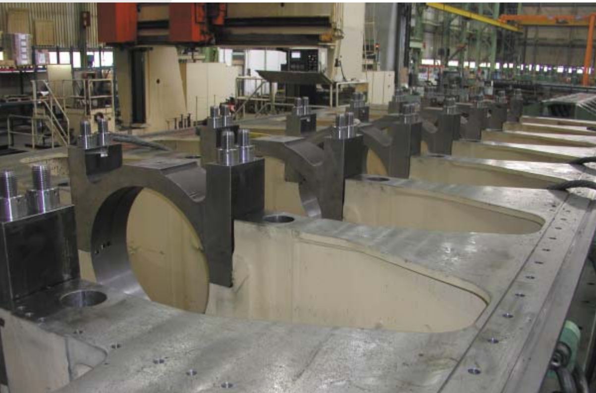
Bedplate of the 7RT-flex60C with main bearing caps in place.
