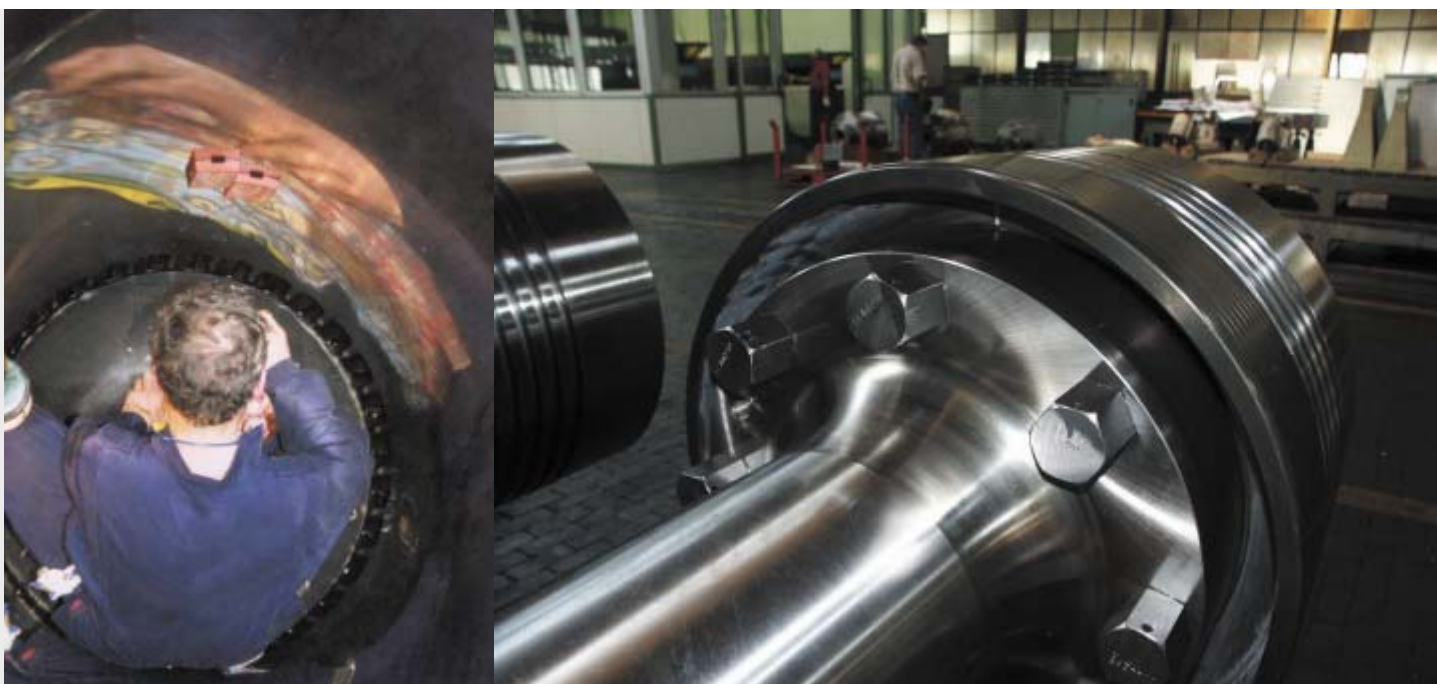
Deep-honed liners soon achieve a mirror surface. Piston of the RT-flex60C.
