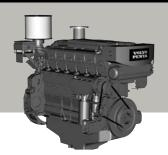
6-cylinder, 4-stroke, direct-injected, turbocharged aftercooled marine diesel engine.
