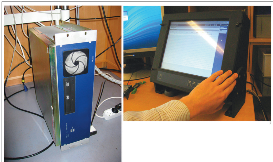
Figure 3: Main Operating Panel (MOP) – Desktop computer
