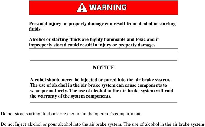
Do not Inject alcohol or pour alcohol into the air brake system. The use of alcohol in the air brake system can cause components to wear prematurely. The use of alcohol in the air brake system will void the warranty of the system components. Alcohol may be injected in certain air compressors in order to prevent moisture from freezing. Consult your Caterpillar dealer for further information.
