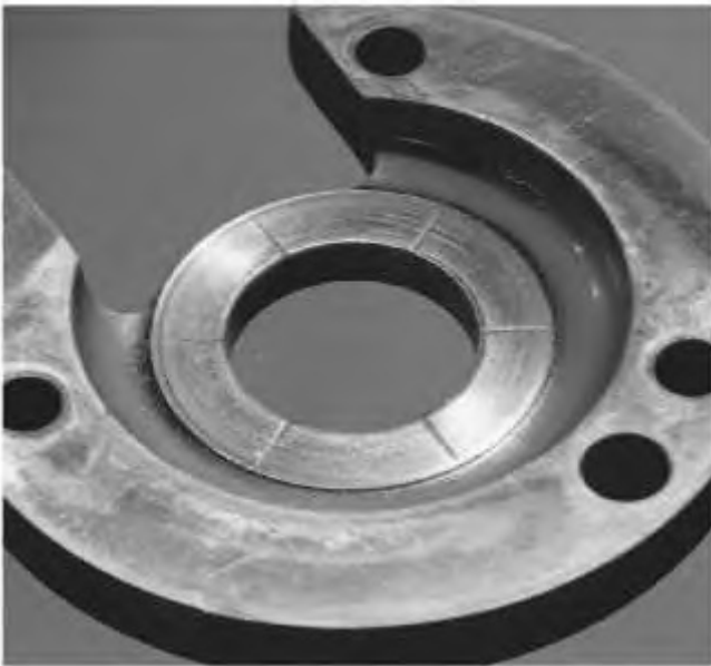
Illustration 40 g02142909 Schwitzer. Thrust bearing surface polished by fine abrasives in the oil.
