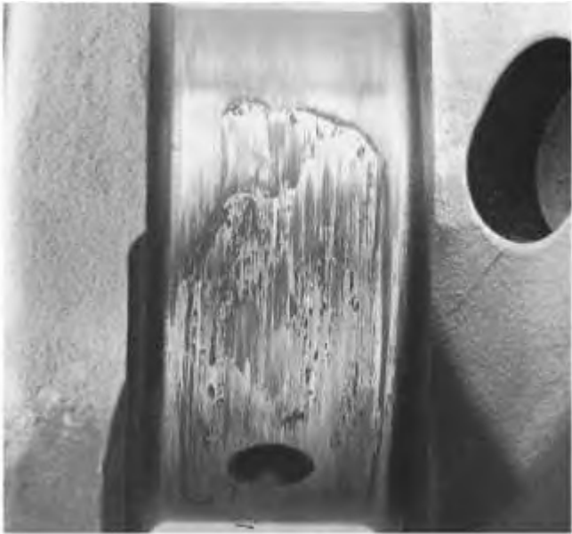
Illustration 20 Result of oil starvation.
