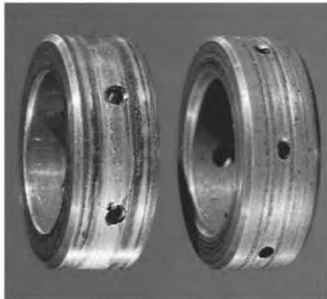
Illustration 28 g02142867 Damage from large abrasive particles in oil. Large, wide grooves around the journal bearings indicate that big particles, such as steel chips, have gone through the turbocharger lubricating oil.
