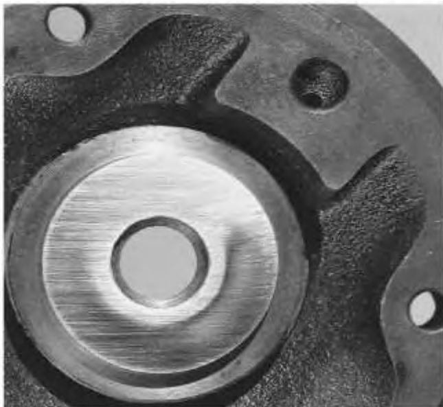
Illustration 35 g02142890 Heat discoloration on inboard side of thrust ring (AiResearch).
