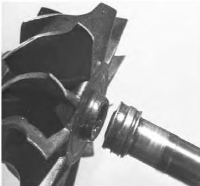
Illustration 34 Shaft broke when contact on turbine hub, due to thrust bearing failure, weakened.
