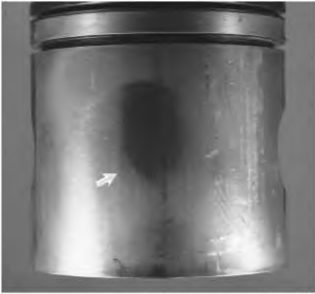
Illustration 24 g02142857 Wear caused by no lubrication for a short period of time.
