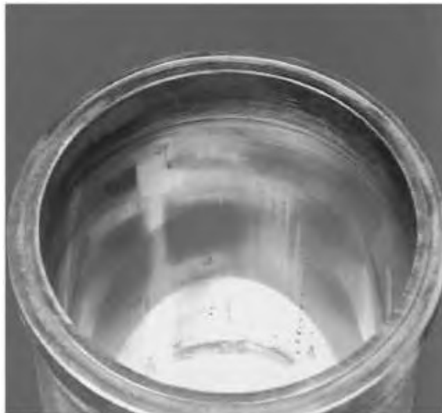
Illustration 25 g02142858 The heavy first and second land deposits indicate the oil can no longer keep the piston clean. The extreme degradation and deterioration of the oil may be due to extended oil change intervals or improper oil performance classification selection.
