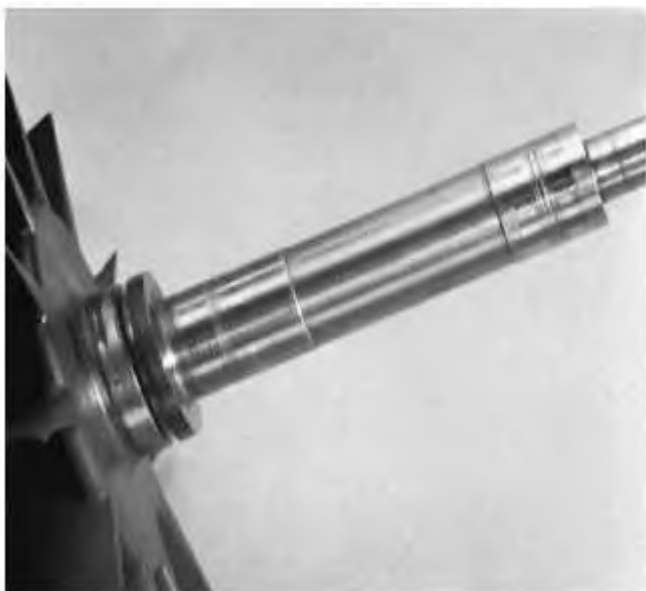
Illustration 36 g02142891 Scratches on both bearing journals ...dirty oil.
