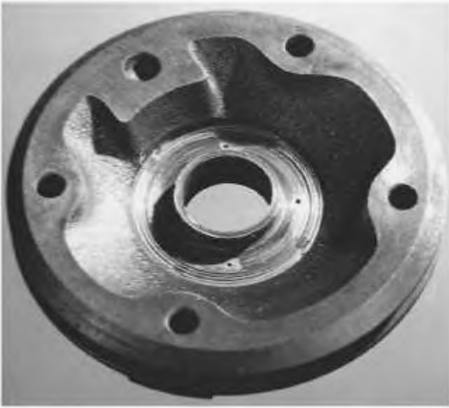
Illustration 39 g02142908 AiResearch. Wear grooves on surface of thrust washers.
