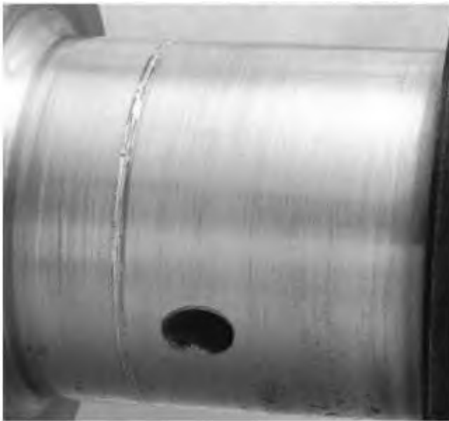
Illustration 21 Deep circumferential scratches shows effects of abrasives embedded in the bearing surface.
