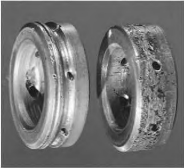
Illustration 27 g02142865 Deep scratches and damage to oil holes on bearings.
