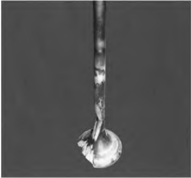
Illustration 41 g02142916 Valve guttering effect caused by excessive deposit formation.
