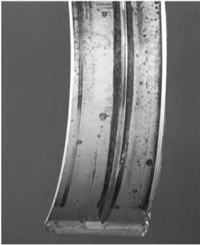
Illustration 16 g02142818 Scratched bearing surface. Notice embedded particles of debris.
