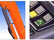
The EB 406 is provided as standard with two travel speeds, including a fast speed to speed up machine travel on the site.
