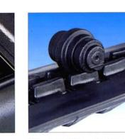
Ride comfort is considerably improved thanks to the profile of the tracks and the alternating position of the guides which provides permanent contact with the rollers.
