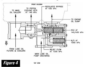
The priority valve regulates oil pressure at the cylinder block main oil gallery rather than at the oil pump. This makes the oil gallery pressure independent of the oil filter and oil cooler pressure drops.
