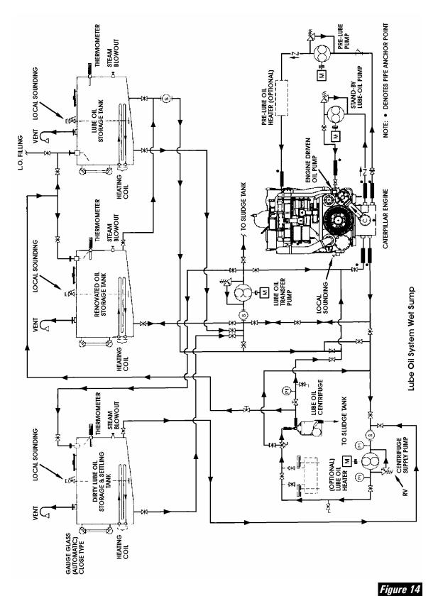
3600/G3600 Lube Oil System - Wet Sump Diagram
