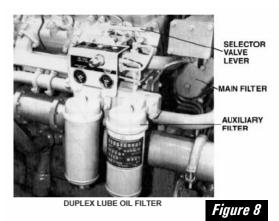
The system provides the means for changing either the main or auxiliary filter elements with the engine running at any load or speed. A filter change indicator is included to tell when to change the main filter elements. A vent valve allows purging of air trapped in either the main or auxiliary system when installing new elements.
