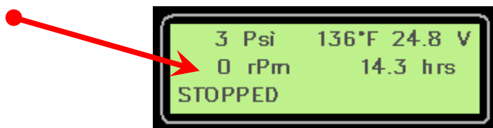
FIGURE 98: ENGINE OVERVIEW SCREEN - STOPPED
