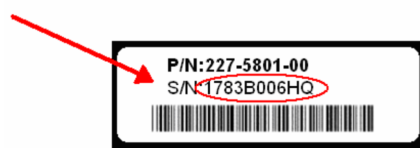
FIGURE 108: SAMPLE CONTROL SERIAL NUMBER ON EMCP 3 GSC LABEL
