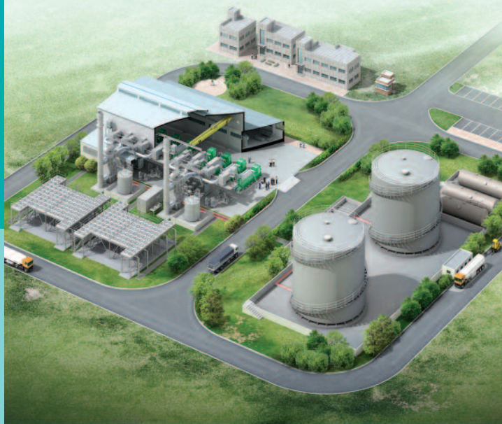
20 MW HiMSEN Engine Diesel Power Plant (9H25/33 x 8 Sets)
