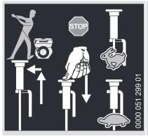
Speed adjustment with connecting rod (additional equipment)
