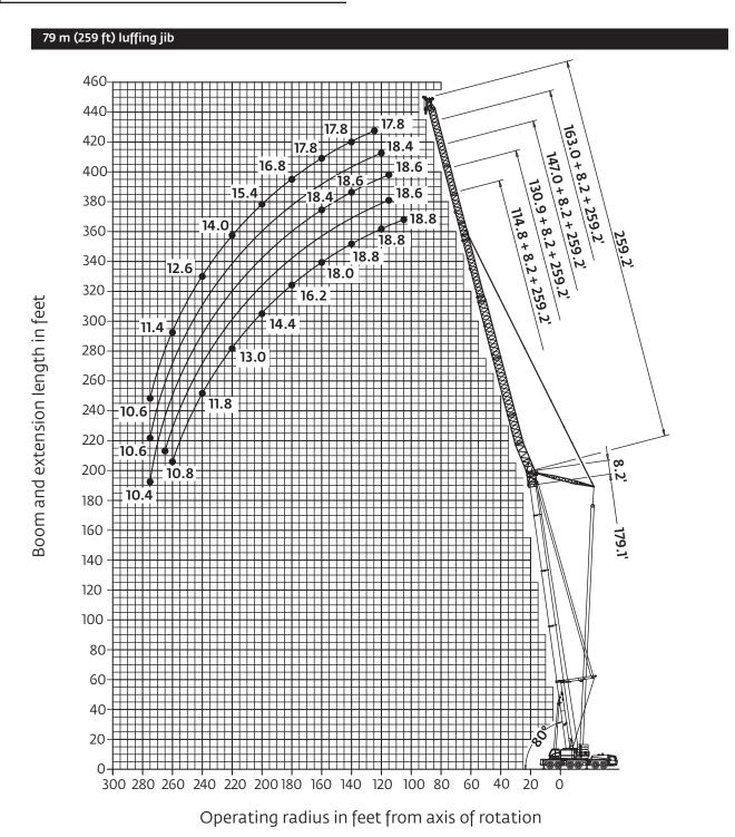
Hook heights shown in the working diagram do not consider loaded boom deflection.
