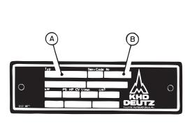
The model type A and the engine serial No. B are given in the engine identification plate.
