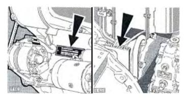
The engine identification plate is mounted to the crankcase.
