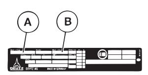
The model type A and the engine serial No. B are given in the engine identification plate.
