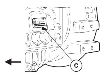
The engine identification plate C is mounted to the crankcase. The serial No. is not stamped into the crankcase.
