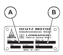
The model type A and the engine serial No. B are given in the engine identification plate.
