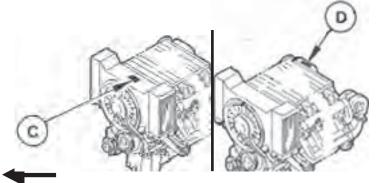
The engine identification plate C is affixed to the oil cooler cover. The engine serial number D is stamped on the gear cover.
