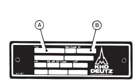
The model type A and the engine serial No. B are given in the engine identification plate.
