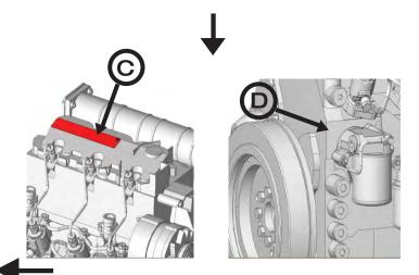
The engine identification plate C is mounted to the valve cover.
