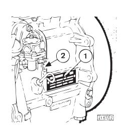
The engine identification plate 1 is mounted to the crankcase.
