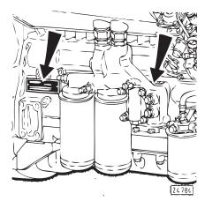
The engine identification plate is mounted to the crankcase at left of the lube filters and in the air cowling. The serial No. is also stamped into
