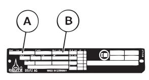
The model type A and the engine serial No. B are given in the engine identification plate.
