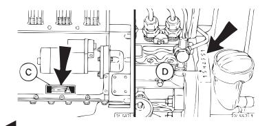
The engine identification plate C is mounted to the crankcase.
