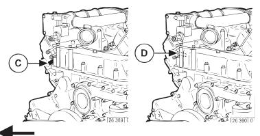
The engine identification plate C is mounted to the crankcase.
