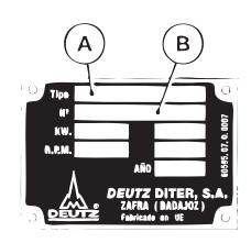
The model type A and the engine serial No. B are given in the engine identification plate.
