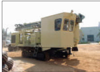
Blast Hole Rig powered by Cummins NT-855-BC
