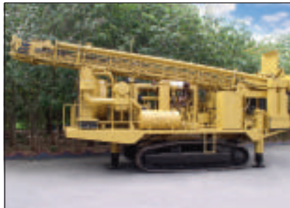
Blast Hole Rig powered by Cummins NT-855-BC
