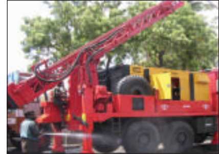
1100 cfm / 300 psi powered by Cummins NTA-855-BC
