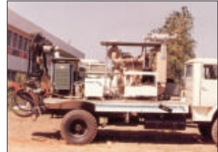
Hydrofracturing Unit powered by Cummins
