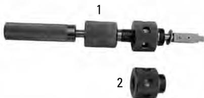
This adapter is used to adapt the 4C-5601 Plunger Compressor to Zexel pumps with M28 threaded plugs.
