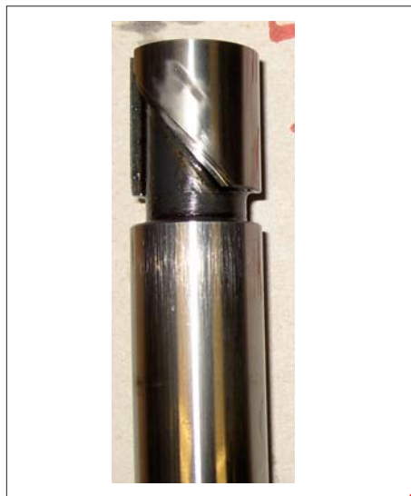
Fig. 23: Plunger with cavitation
