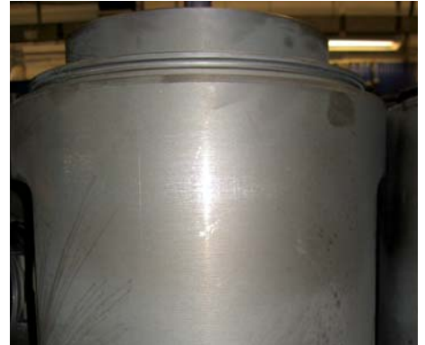
Fig. 16: Piston skirt can continue service after reconditioning of the piston steel top
