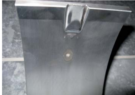
Fig. 21: Main bearing no. 2 - Cavitations mark visible
