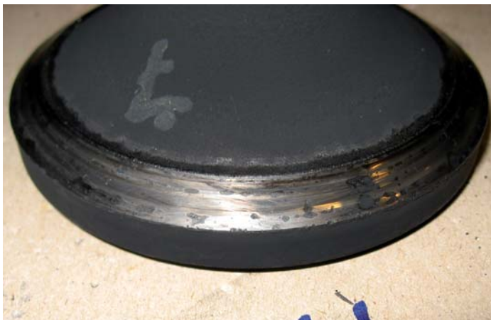
Fig. 13: Exhaust valve after 46,300 hrs of operation
