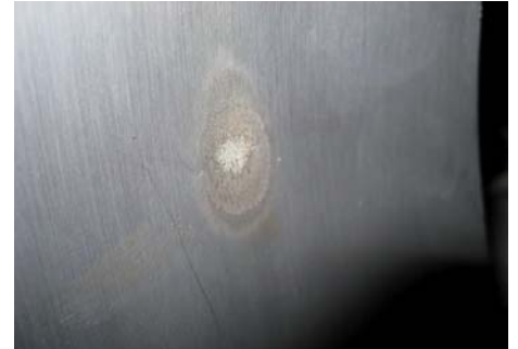
Fig. 22: Main bearing no. 2 – Close-up of the cavitation marks. Visible at the ends of the oil grooves
