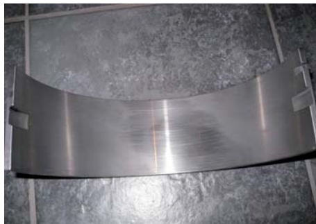
Fig. 17: Main bearing no. 1 after 46,300 hrs of operation
