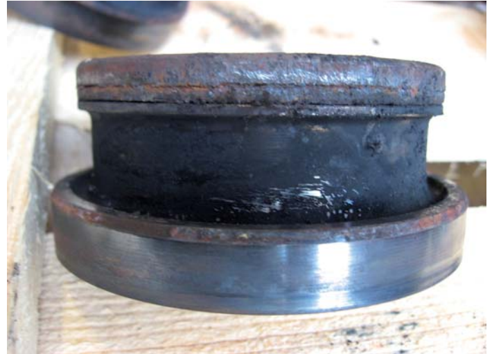
Fig. 12: Exhaust seat ring – corrosion-damaged due to inadequate cooling water inhibitor
