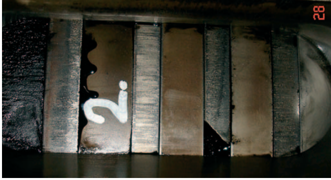
Fig. 6. Totally scuffed unit. Lubrication should be increased to maximum until overhaul is convenient with regard to the schedule of the ship. Due to the friction heat developed, the piston rings get hardened, and the wear rate of the liner increases significantly. However, the hardening protects the rings, which is why operation may be continued safely until next convenient port stay.
