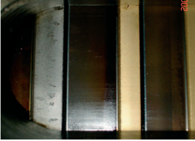
Fig. 4. Unit with micro-seizures on the top ring as a result of metal-to-metal contact. Should be counteracted by temporarily increased lubrication. It is important to lower the lubrication to normal as soon as the active mz-attack is stopped. Note that old, not active, mz-marks remain visible long after the attack has stopped and do not call for increased lubrication.
