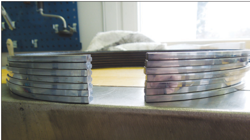
Fig. 17: Piston ring condition after more than 20,000 hrs. in service (7L23/30H)
