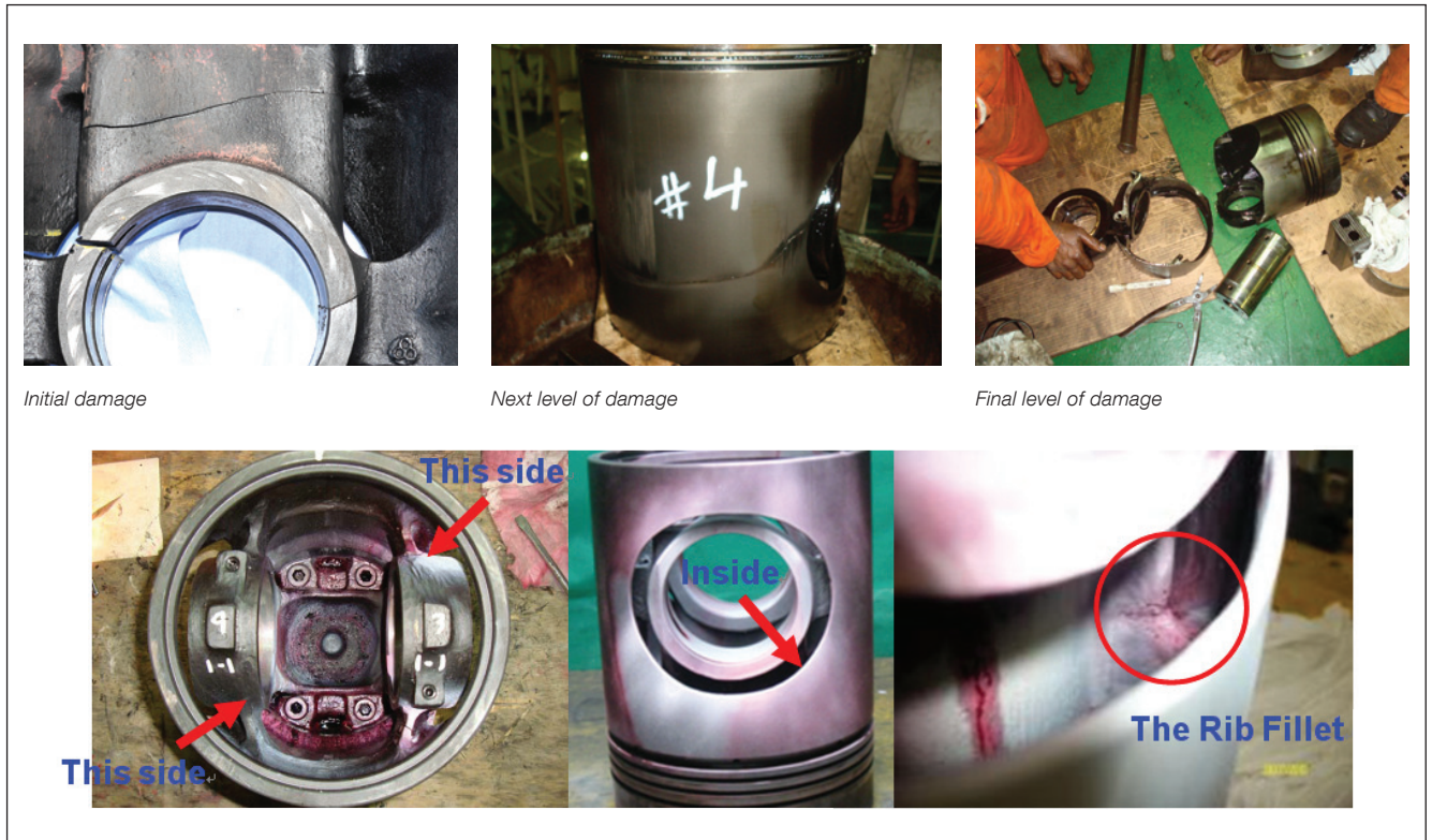
Fig. 9: Cracked pistons on L23/30
