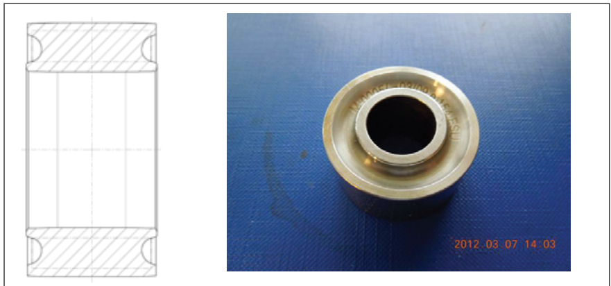
Fig. 20: L28/32 soft shoulder cam design
