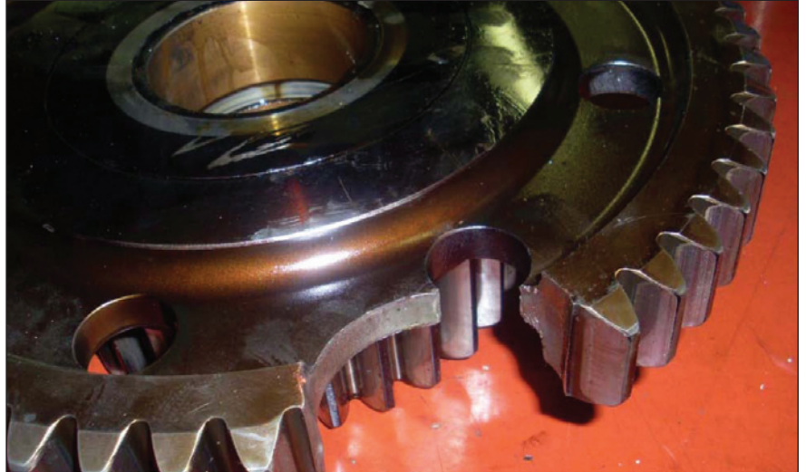
Fig. 12: Broken gear wheel from L27/38
