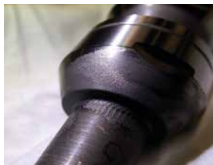
Fig. 58: Cavitation on PEVA slide version I
