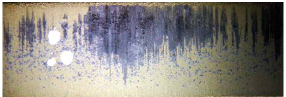
Fig. 28: Piston ring running surface where the hard coating (CM1) has penetrated the running-in alucoat
