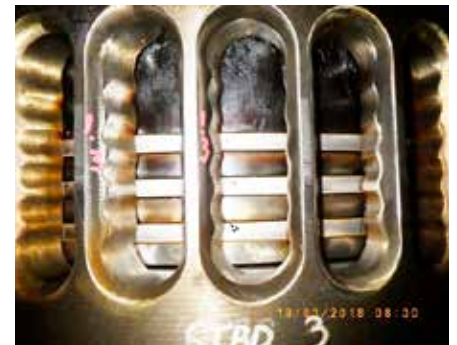
Fig. 11: The continuous operation on low-sulphur fuel and the alternating use of high- and low-BN cylinder oil give sufficient detergency
