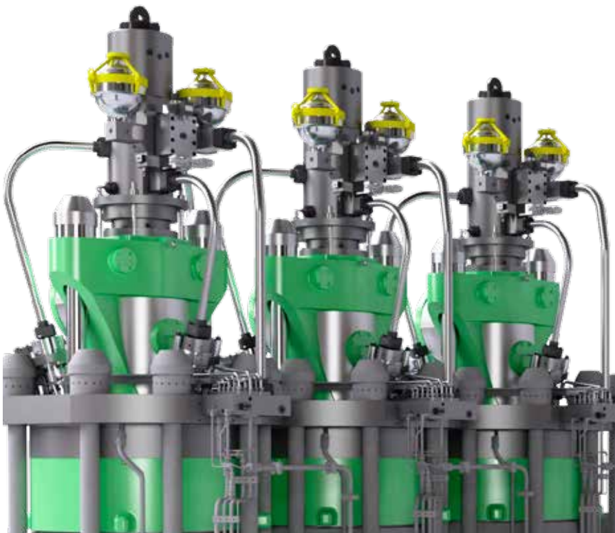
Fig. 66: Three units with TCEV/FBIV on an 8G95ME-C9.5 engine
