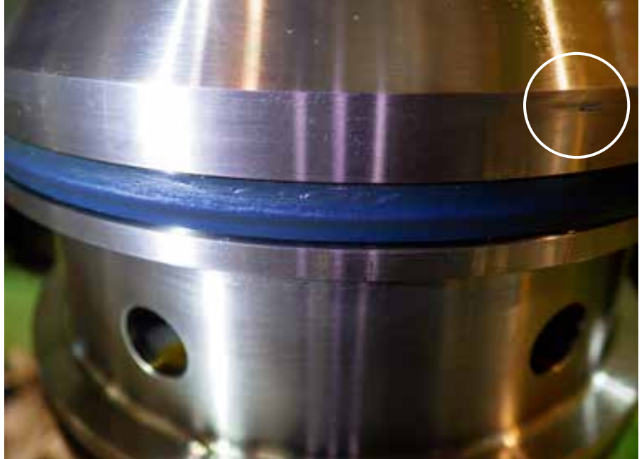
Fig. 64: Imprint from actuator slide pressure piece
