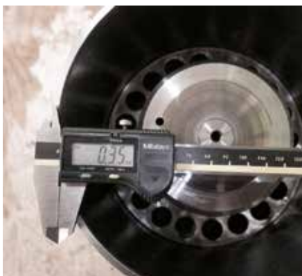
Fig. 61 Imprint from actuator slide pressure piece
