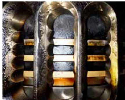
Fig. 10: The continuous operation on low-sulphur fuel and the use of low-BN cylinder oils give insufficient detergency
