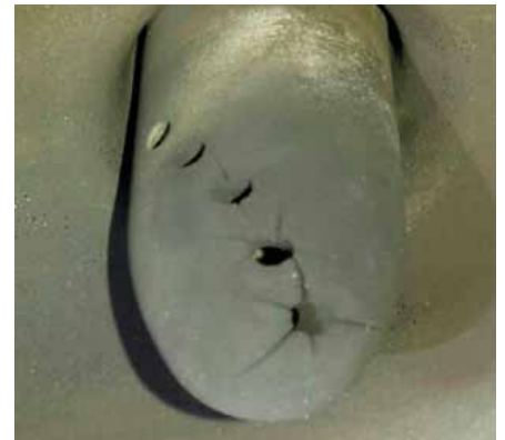
Fig. 7: Cracks in the GIV nozzle
