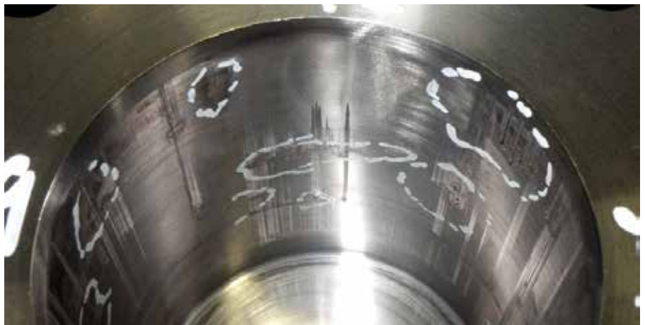
Fig. 55: Fretting inside the measuring cone
