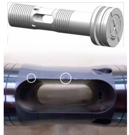
Fig. 67: Inlet hole of suction valve
