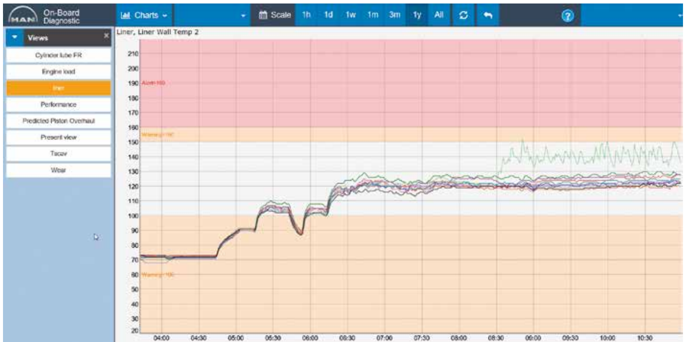
Fig. 47: OBD liner wall graph, during scuffing
