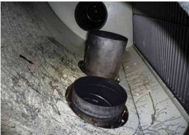
Fig. 43: Mixing chamber on a 6G70ME-C9 (LSFO operation)
