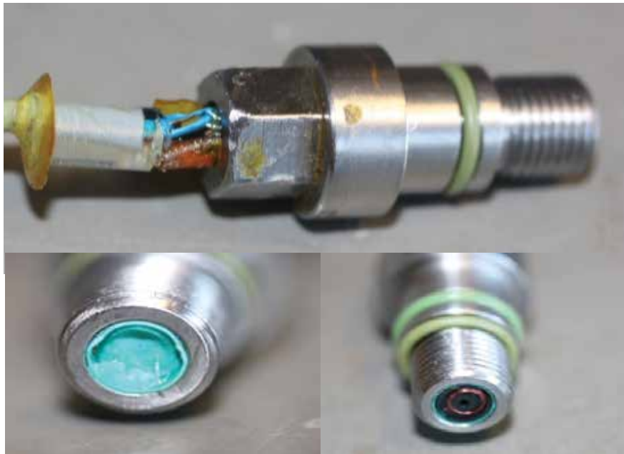
Fig. 31: Mechanical damage on Pepperl & Fuchs.
