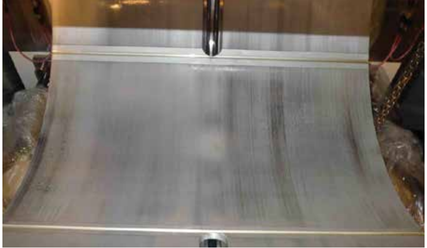
Fig. 12: 7G80ME-C9.2 – crosshead bearing after sea trial
