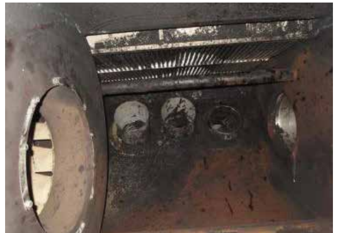
Fig. 44: Mixing chamber on a 6S80ME-C9 (HSFO operation)
