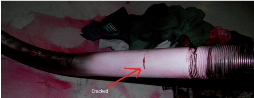
Fig. 34: Cracked central high-pressure fuel pipe of the hose type
