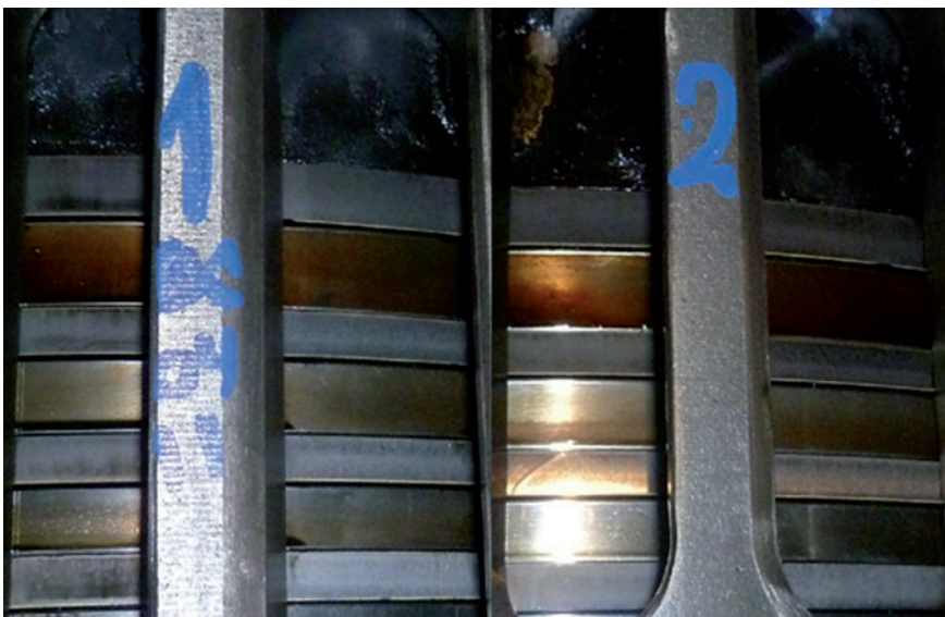
Fig. 23: 6S46MC-C unit with POP ring pack
