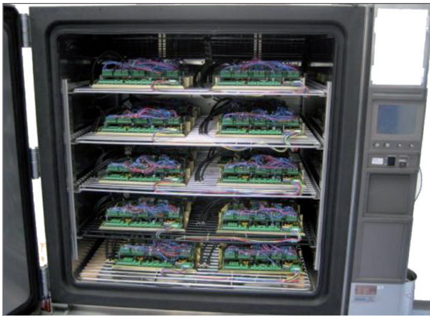
Fig. 1: Burn-in test of MPCs
