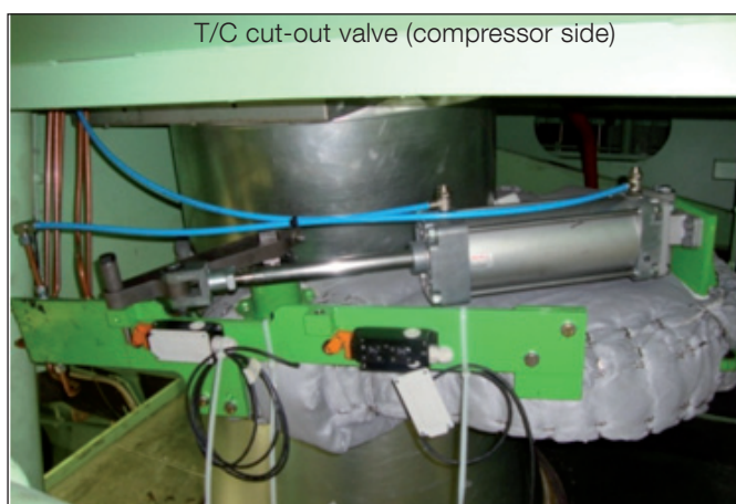
Fig. 8: Swing gate valve for flexible T/C cut-out
