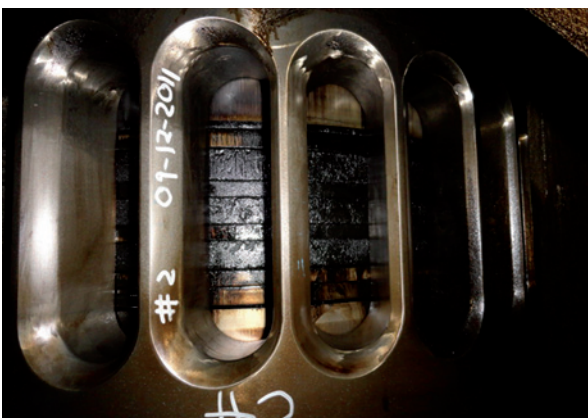
Fig. 28: S80ME-C9: Collapsed/broken piston rings
