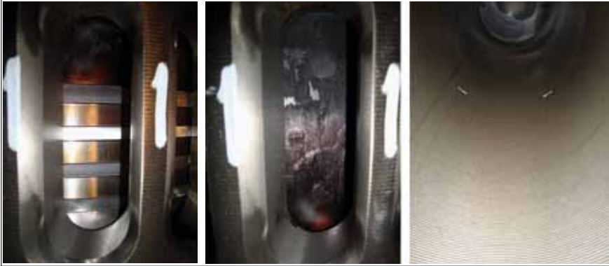
Fig. 24: Scavenge port inspection
