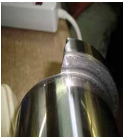
Fig. 4: Piston collar breakage
