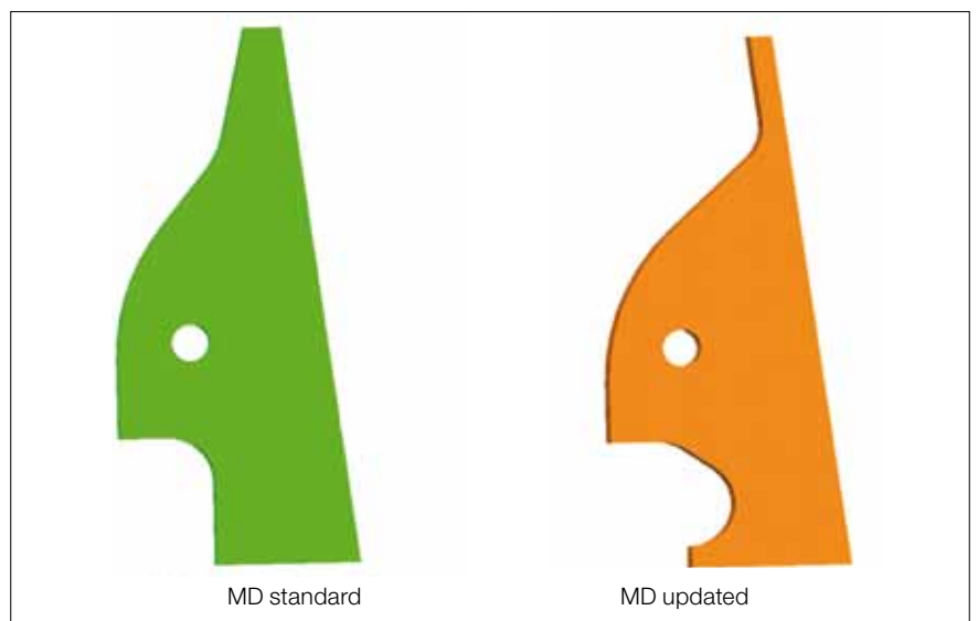
Fig. 37: Lifting bracket cracks: design update
