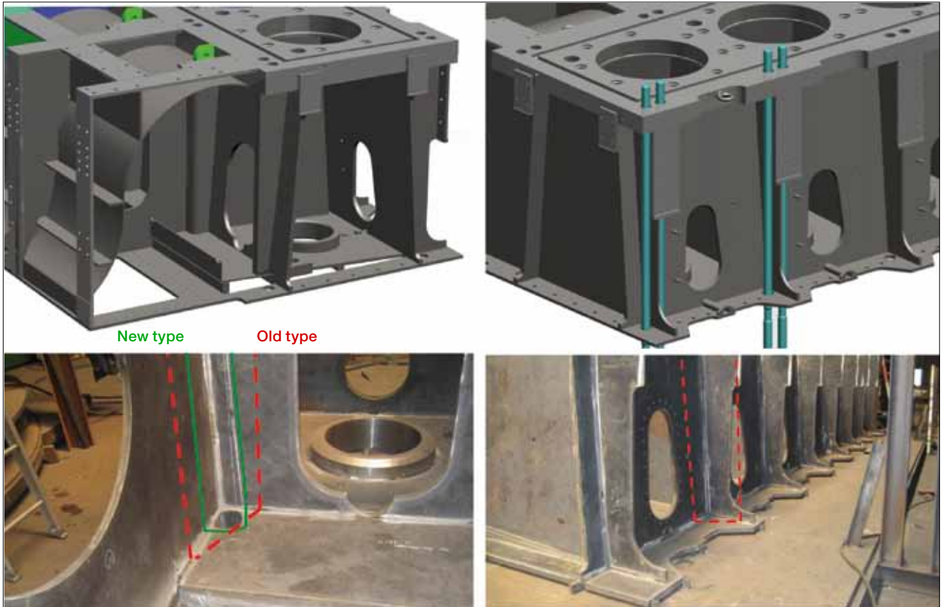
Thin, bent stay bolt cover in exhaust side. New type/old type Fig. 40: Welded cylinder frame: old and new type stay bolt cover designs
