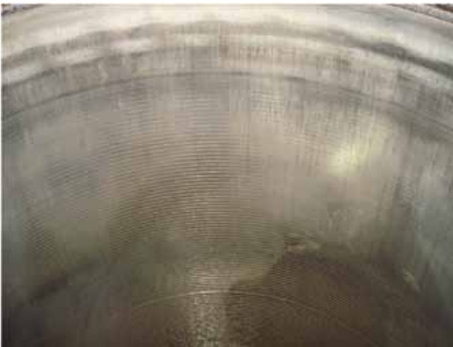
Fig. 18: Top of liner after 3,800 hrs.
