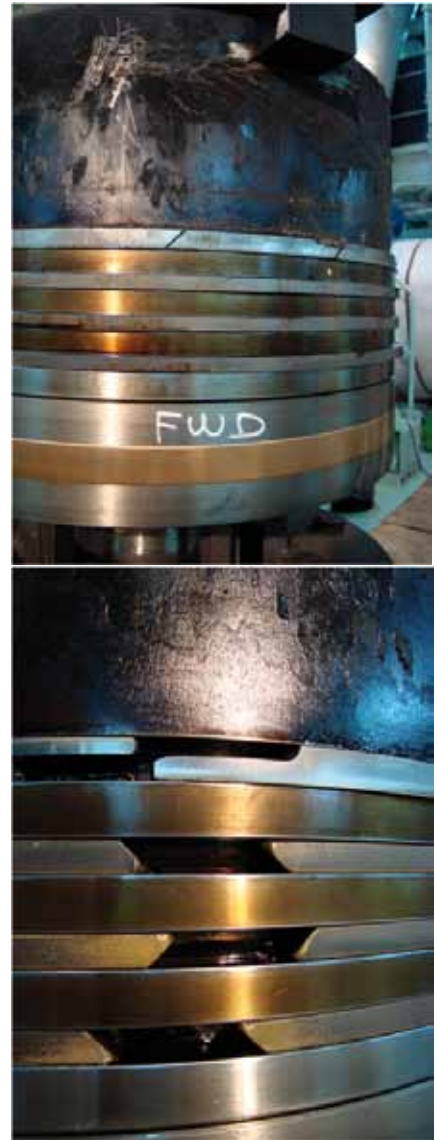
Fig. 26: ME-B9 piston after 4,000 hrs
