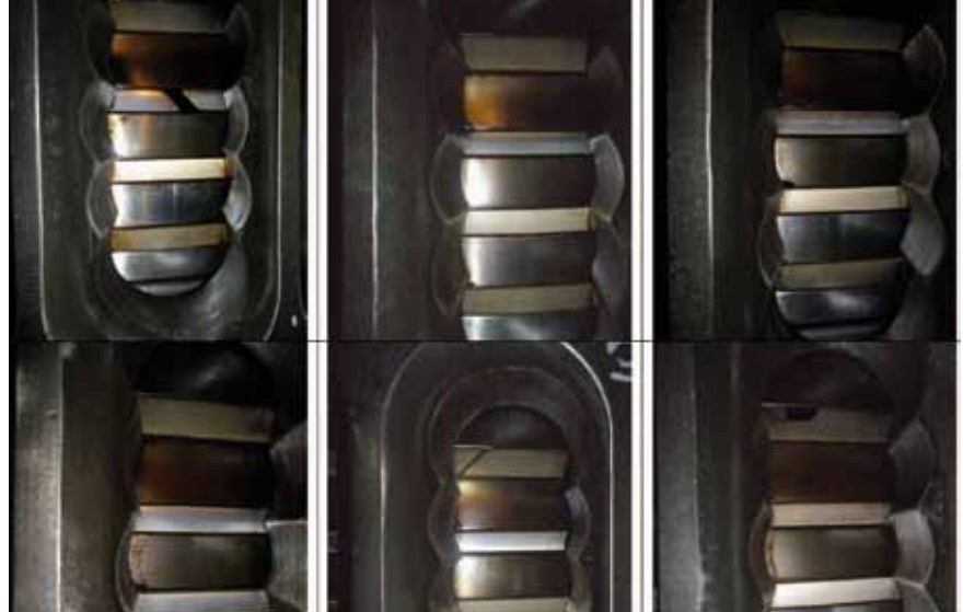
Fig. 15: Piston ring condition
