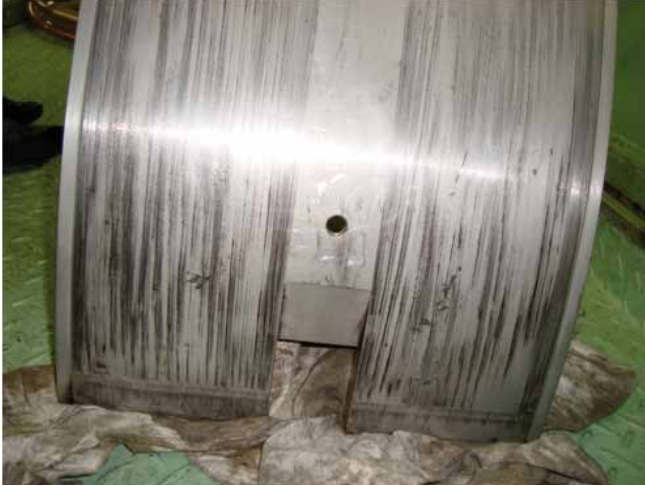
Fig. 22: Upper main bearing shell backside
