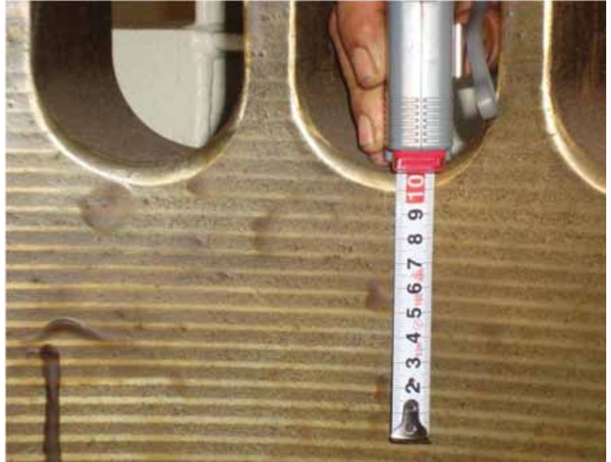
Fig. 31: Cylinder liner quality: insufficient plateau honing
