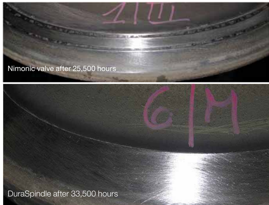
Fig. 44: W-seat in combination with Nimonic spindle and DuraSpindle on an S60MC
