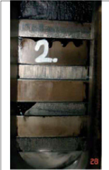
Fig. 8.28: Totally scuffed unit. Lubrication should be increased to maximum until overhaul is convenient with regard to the schedule of the ship. Due to the friction heat developed, the piston rings get hardened and the wear rate of the liner increases significantly. However, the hardening protects the rings, which is why operation may be continued safely until next convenient port stay.
