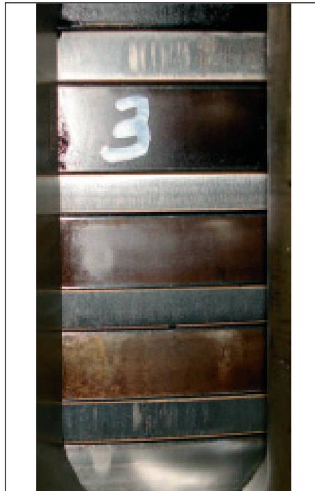
Fig. 8.29: Unit with micro-seizures on the top and bottom rings as a result of metal-to-metal contact. Should be counteracted by temporarily increased lubrication. It is important to lower the lubrication to normal as soon as the active mz-attack is stopped. Note that old, not active, mz-marks remain visible for a long time and do not call for increased lubrication.
