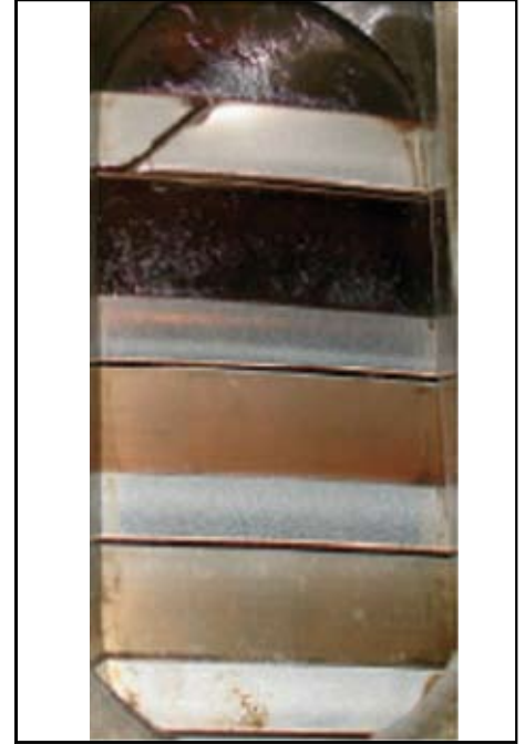
Fig. 8.27: Unit with 23,500 hours without piston overhaul. Note that most of the rounding is still intact, indicating that only 1/4 of the wear potential is used. Further, the measurements above from the same unit show that only 1/2 of the ring groove wear potential is used, and the rate of burnings on the piston top is insignificant. Consequently, overhaul of that unit is not needed at this stage.
