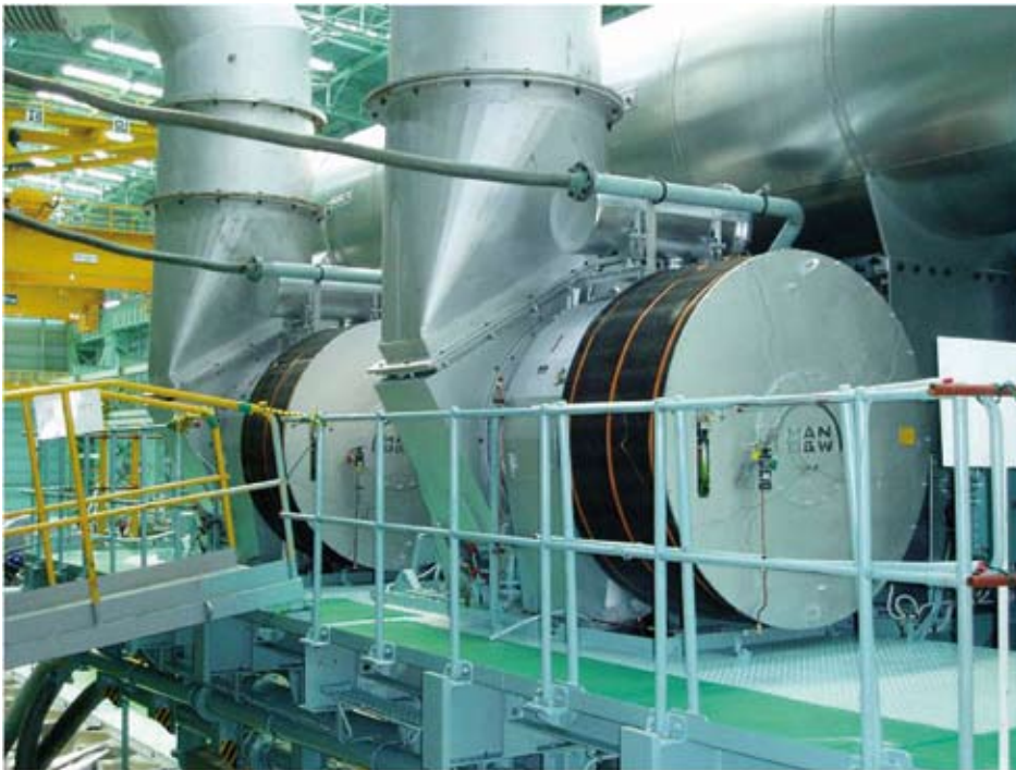
Fig. 8.39: Modern turbocharger enabling more than 30,000 hours between major overhauls
