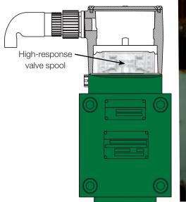
Fig. 14: ELVA valve, location and high-response valve spool
