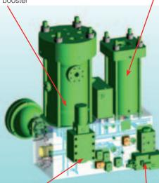
FIVA valve Integrated Alpha Lubricator Fig. 9: Hydraulic Cylinder Unit (HCU)
