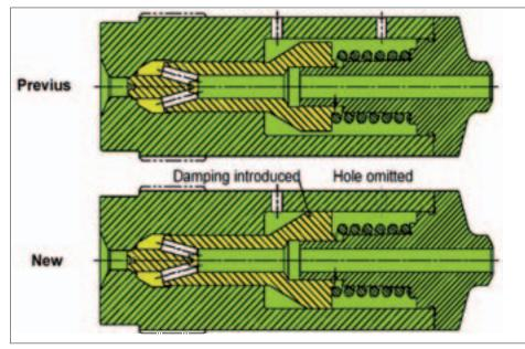
Fig. 27: ME-fuel injector: internal damping applied at non-return valve
