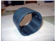
Fig. 29 Exhaust valve high pressure pipe: Chafing guard installed between highpressure pipe and protective tube
