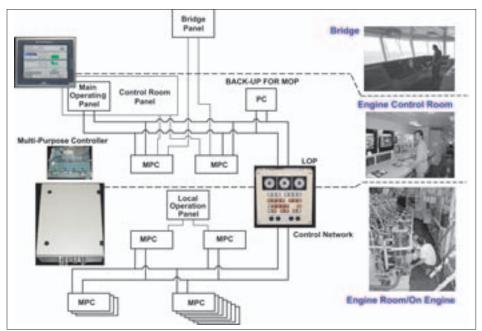
Fig. 7: Engine Control System (ECS)
