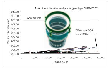
Fig. 47: 6S90MC-C, cylinder liner wear
