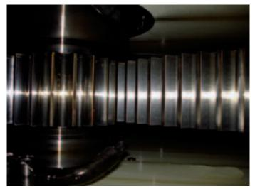
Fig. 36: 12K98ME, gearbox for engine driven hydraulic pumps, excellent condition of gears after 10,762 hours
