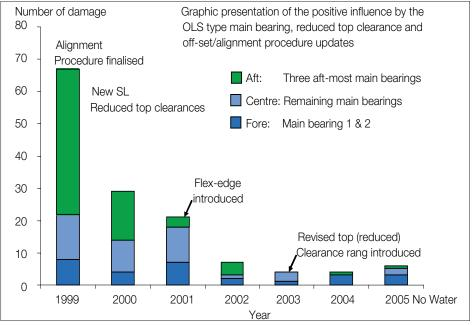
Fig. 55: Main bearing damage statistic
