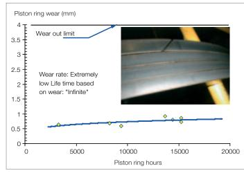
Fig. 44: Piston ring wear measurements, prototype 6S90MC-C (M/T Maria A. Angelicoussis)
