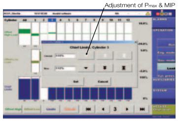
Fig. 4: Easy engine balancing/adjustability
