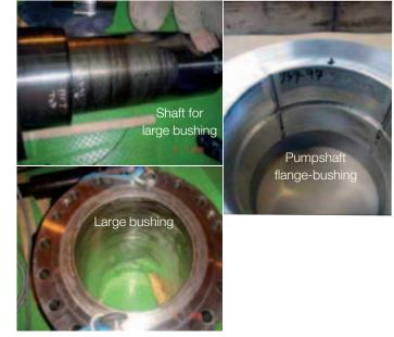
Fig. 31: HPS gearbox: Failed bushings/bearings
