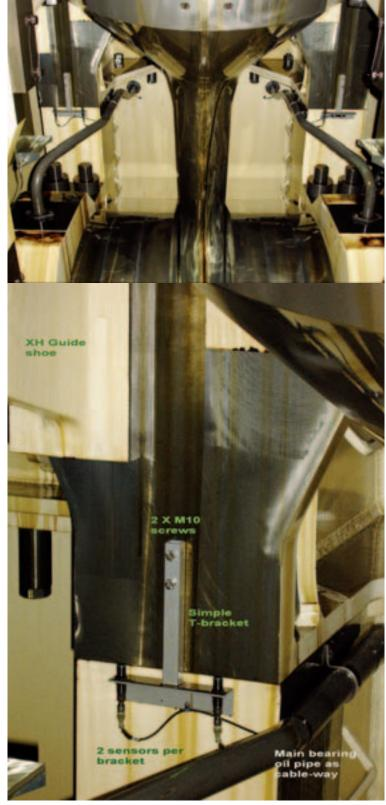
Fig. 61: BWM installation on a K98MC-C
