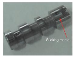
Fig. 15: ELVA valve, sticking high-response valve spool
