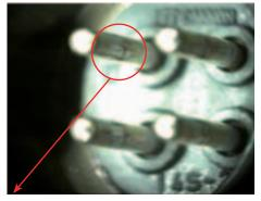
Fig. 24: Scratch marks on connector for exhaust valve feed back sensor
