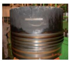
Fig. 11: 12K98ME prototype engine, piston inspected after 10,762 running hours
