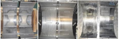
Partially corroded overlay, not yet scuffed
