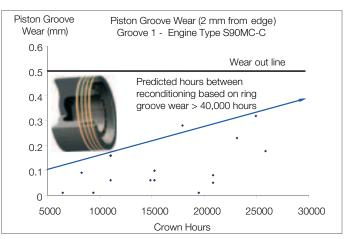
Fig. 49: 6S90MC-C, Piston ring groove wear
