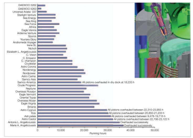
Fig. 43: Fleet of VLCCs equipped with 6S90ME-C/MC-C
