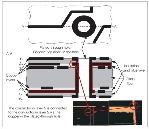
Fig. 38: PCB, broken copper layers
