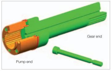
Fig. 34: Pump safety shaft, initial design
