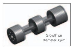
Fig. 20: FIVA valve, growth of main spool
