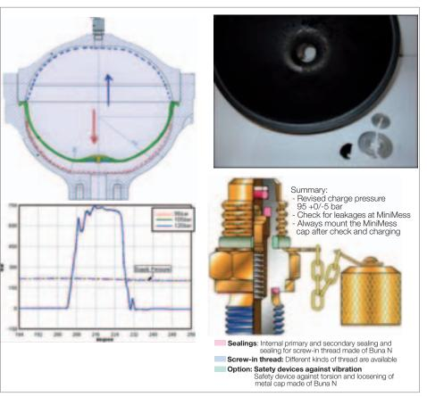
Fig. 25: Maintenance of accumulators
