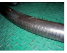
Fig. 28: Exhaust valve high pressure pipe: Serious dent marks has been observed
