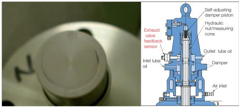
Fig. 23: Exhaust valve feedback sensor
