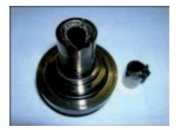
Fig. 26: ME fuel injector: breakage of cut-off shaft and non-return valve
