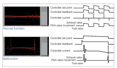
Fig. 21: Uncontrolled feedback signal due thermal overload of FIVA electronics FIVA valve, growth of main spool
