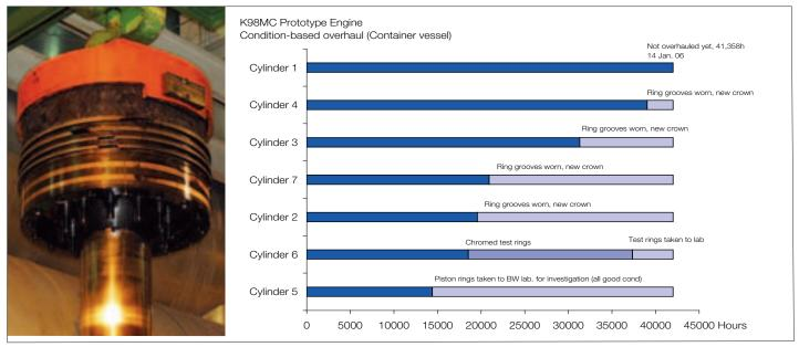
Fig. 54: 7K98MC, condition-based overhaul piston No. 1 overhauled first time after 42,500 hrs
