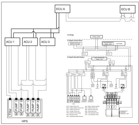
Fig. 40: ME-system, control diagram (initial version)
