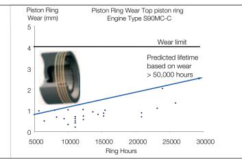
Fig. 48: 6S90MC-C, Piston ring wear
