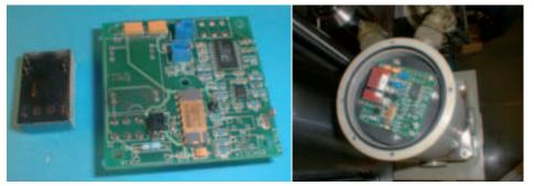
Fig. 12 : ELFI valve, DC-DC converter coming off due to vibration of PCB
