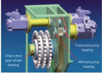
Fig. 30: HPS gearbox: Position of bushings
