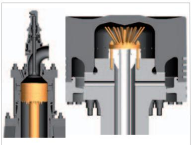
Fig. 53: Piston cooling insert
