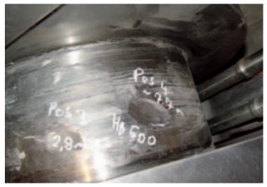
Fig. 60: Main bearing journal as result of steel-to-steel contact
