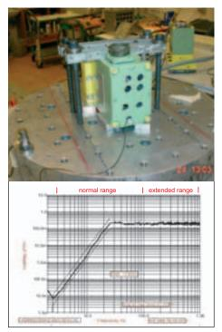
Fig.19: Control valve, extended vibration testing
