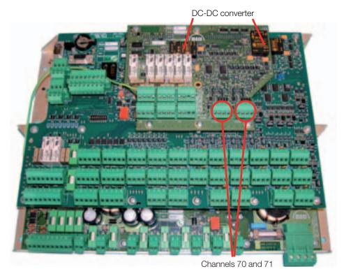
Fig. 37: MPC board, failure of channels 70 & 71
