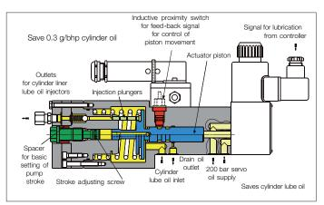
Fig. 5b: System integration, example: Alpha Lubricator
