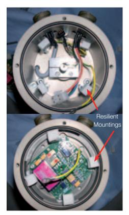
Fig. 13: ELFI valve, PCB secured by resilient mountings
