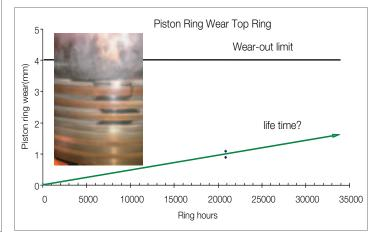
Fig. 45: Piston ring wear measurements, 6S90MC-C (M/T Kos)
