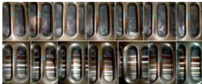
Fig. 11: 7S50ME-C, cylinder condition after 10,717 running hours
