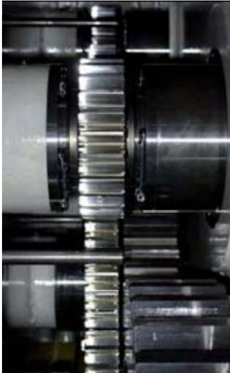
Fig. 32: 7S50ME-C, gearbox for engine-driven hydraulic pumps
