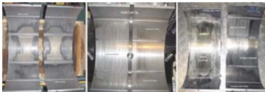
Partially corroded overlay, not yet scuffed Overlay completely corroded, away, Ni 100% exposed, partial scuffing between Ni-layer and pin Overlay completely corroded, away, partly scuffing between Ni-layer and pin, partly steel-to-steel
