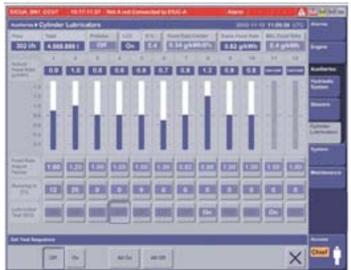
Fig. 5A: System integration example: Alpha Lubricator
