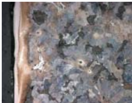
Fig. 53: Piston ring with 'white layer'
