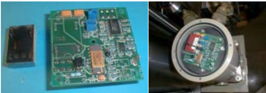
Fig. 14: ELFI valve, DC-DC converter coming off due to vibration of PCB
