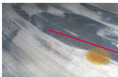
S90MC-C crosshead # 6 (3,500 hours) before dressing up. Note that the lead overlay apparently has a tendency of non-conformity. In this case the problem is only cosmetic
