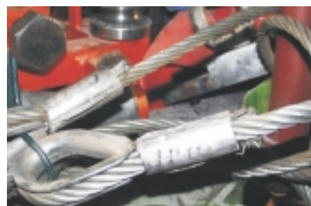
Fig. 21: Wire ends with strands of wire sticking out
