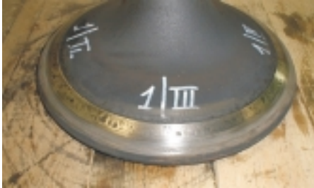
Fig. 15: Nimonic valve normal condition, after 11,500 running hours
