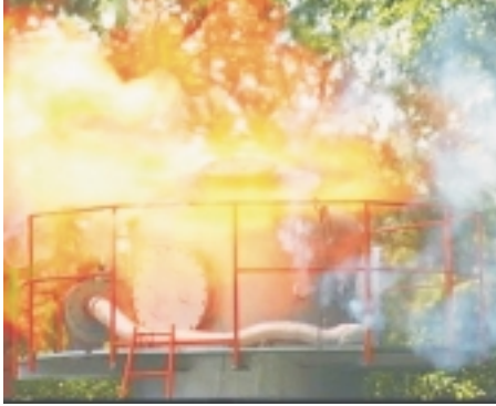
Fig. 23: Testing of a non-functioning crankcase relief valve
