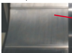
S90MC-C crosshead # 6 (3,500 hours) after dressing up
