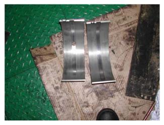
Fig. 15: Connecting rod bottom-end bearing dismantled and cleaned before dye checking.
