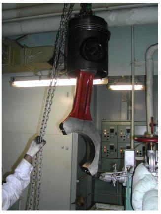
Fig. 7: Piston with new rings ready for installation
