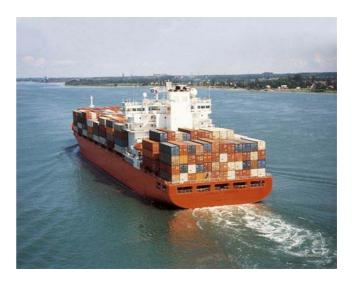
Fig. 1: CP Ships '96- and '95-built 2200 TEU container carriers *M/V Canmar Courage* and *M/V Canmar Fortune* – supplied by Korean Daewoo Heavy Industries
