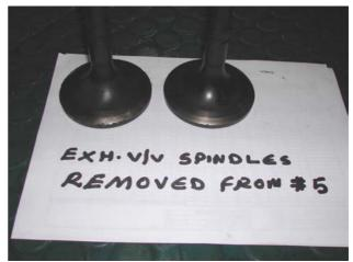
Fig. 3: Exhaust valve spindles
