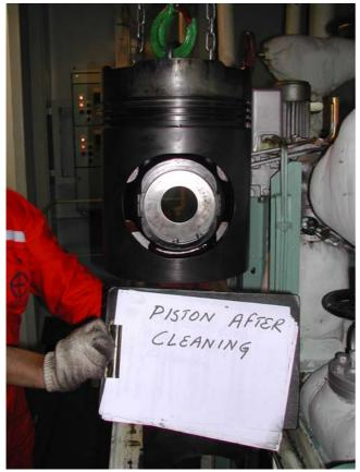
Fig. 6: Piston after cleaning
