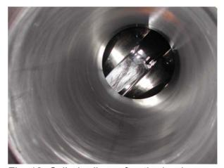
Fig. 12: Cylinder liner after the honing process
