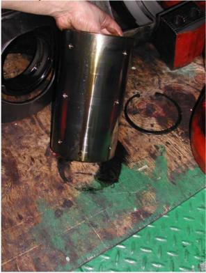
Fig. 13: Piston pin removed for calibration
