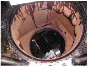
Fig. 8: Cylinder liner in block before removal Fig. 9: Cooling water space – liner removed
