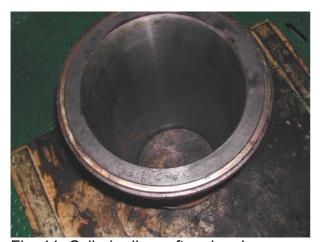
Fig. 11: Cylinder liner after cleaning
