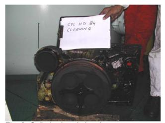
Fig. 2: Cylinder head cleaning
