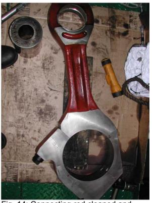
Fig. 14: Connecting rod cleaned and assembled for calibration measurements
