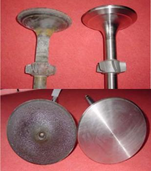
Figure 15 a/b: Nimalike spindle before and after remanufacturing
