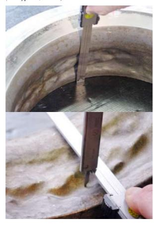
Figure 06: Low temperature corrosion of bottom piece (RTA-type after 28,420 hrs)
