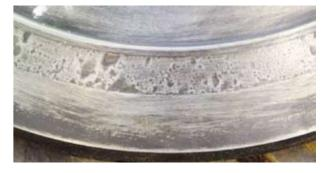
Figure 03: Typical dent marks of the seat of a valve spindle (MC60-type Nimonic after 8,300 hrs)
