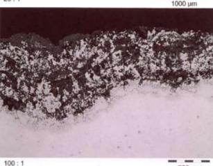
Figure 09: Micro cuts of Nimonic with high-temperature corrosion.
