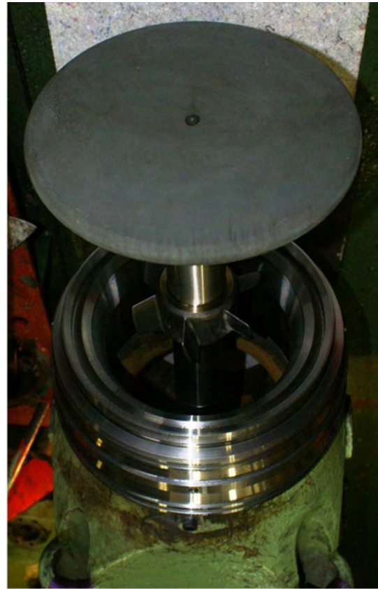
Figure 11 – Picture of the MC50 Nimonic 80A valve spindle with 600 \mu m thick CrystalCoat coating on the valve face and outer diameter, prior to initial engine installation.
