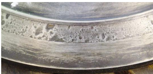
Figure 3: Valve spindle with extensive evidence of dent marks [6].
