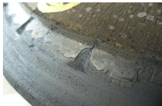
Figure 4: Valve spindle with extensive "glassy-deposits" and beginning of blow-byes.
