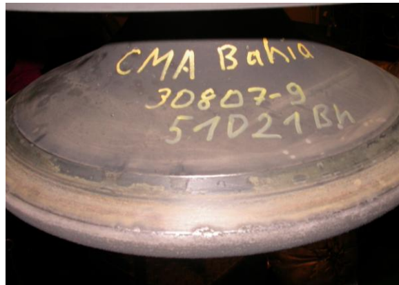
Figure 14: Photograph of valve spindle seat surfaces after 37,505 hours.
