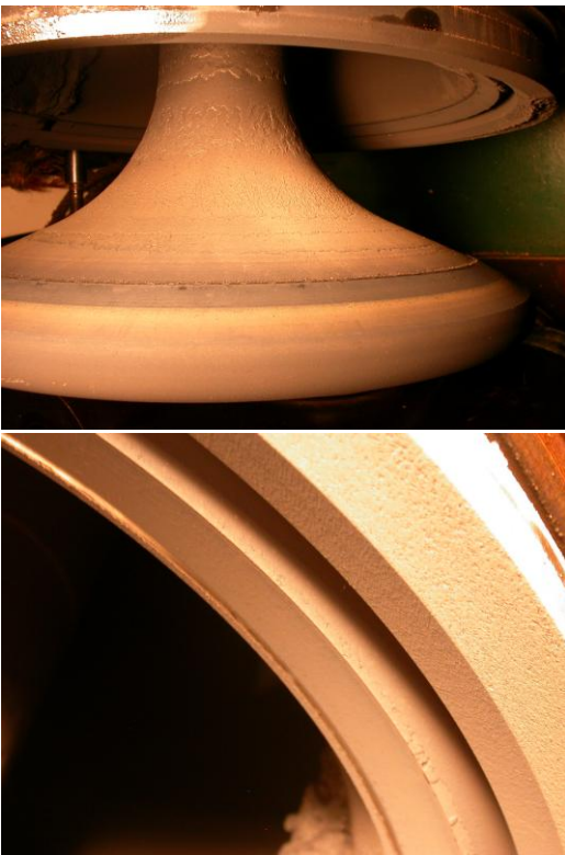
Figure 11: Photographs of the valve spindle and seat ring surfaces after 9,100 hours [6].
