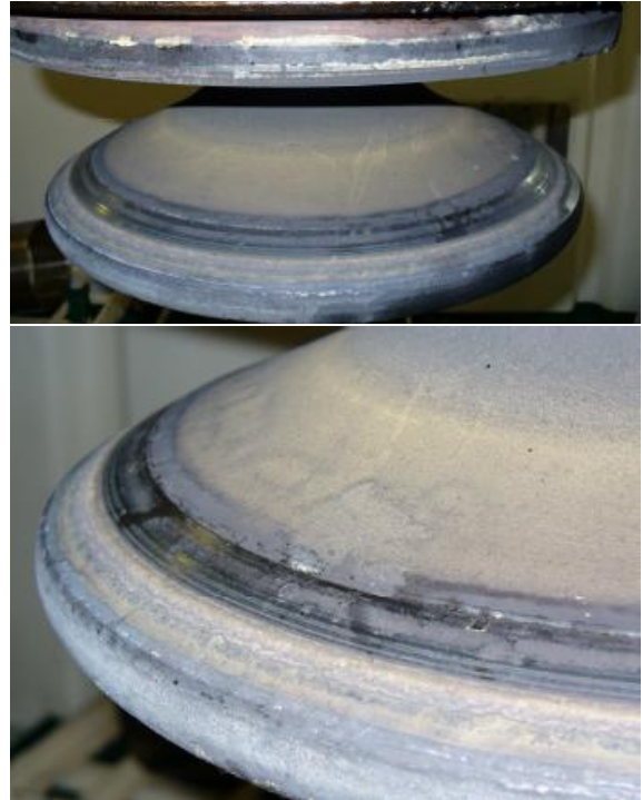
Figure 12: Photograph of the valve spindle and seat ring surfaces after 16,647 hours [6].
