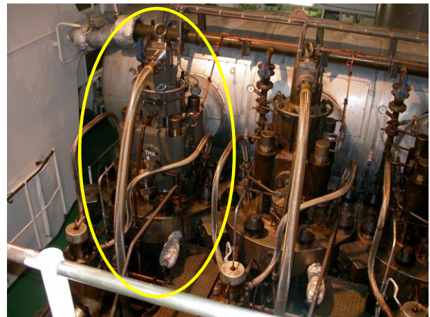
Figure 9: Cylinder #1 of the MAN-B&W 7L70MC engine on the "MV Libra Buenos Aires / CMA CGM Bahia" [6].
