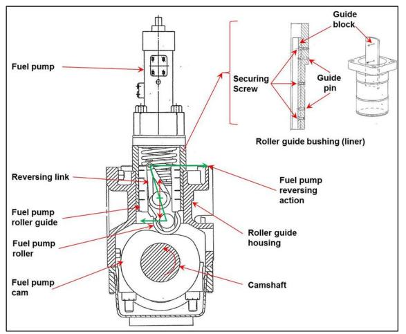
Figure 9: MAN B&W fuel pump, cam, roller, guide and reversing arrangement
