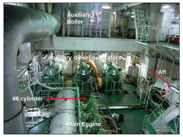
Figure 8: ID Integrity engine room layout
