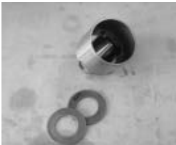
Tappet disassembled and FIC adjust shim.
