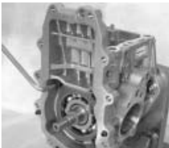
Remove the retainer, (bearing) fastening bolt.
