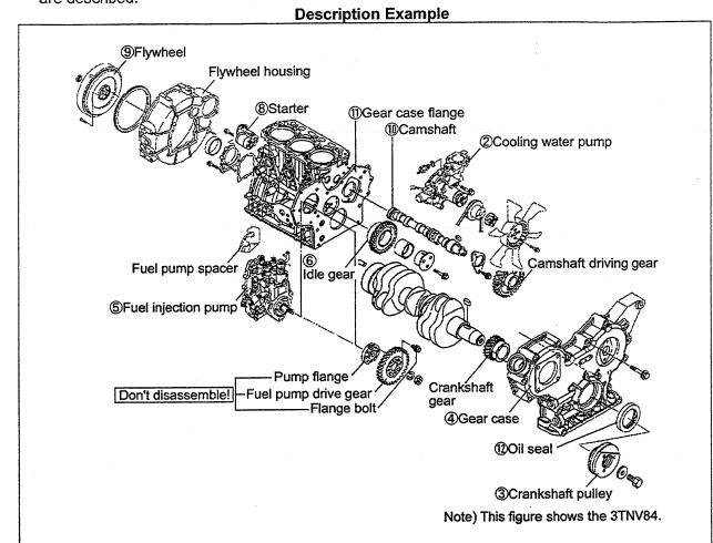
The job contents are described in the disassembly procedure for Nos. not shown in the illustration.
