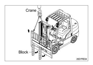
② While supporting lift chains, remove nuts and split pin from the anchor bolt.
