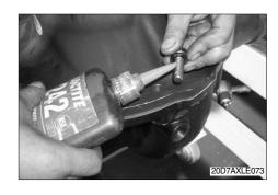
**(6)** Temporarily assemble bolt and confirm torque.
