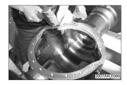
② Spread sealant on the installation surface of carrier.
