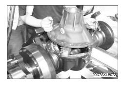
⑤ Spread loctite #277 on the spring washer bolt.
