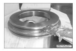
④ Fix piston into drive axle housing.
