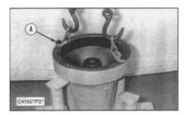
**8.** Fasten Tooling (A) and a hoist to the axle shaft housing as shown. Put slight lifting tension on the axle shaft housing.
