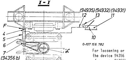
The illustrations show the tightening device when tightening the piston rod screw 2. For the loosening the jack holder 5 has to be fitted to the opposite side at 'L' and the jack has to press on the other side of the spanner 7.
