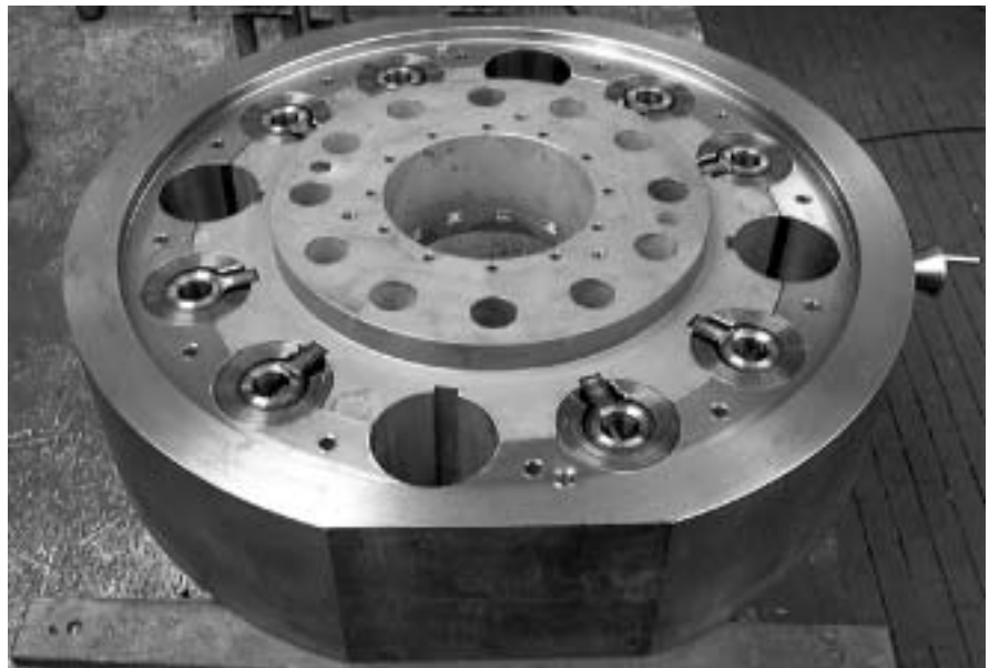
Figure 6. Torsional vibration damper, with some spring assemblies in place
