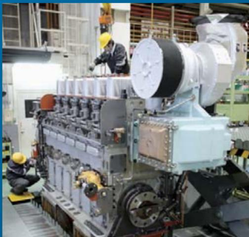
Large Diesel Engine Assembly Process
