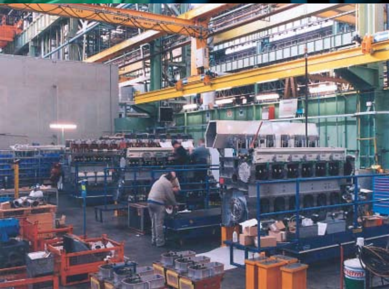
Main assembly shop for Wärtsilä 26 engines in Trieste, Italy.
