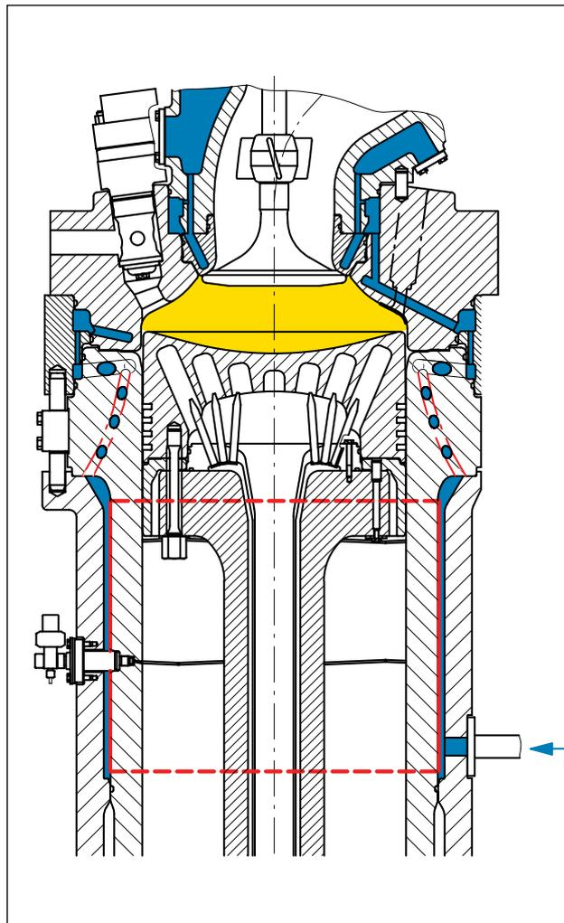
The cylinder liner is bore cooled as well. Great effort was made on the layout of the surface temperatures of the liners (Fig. 24) and on the stress and strain calculations.
