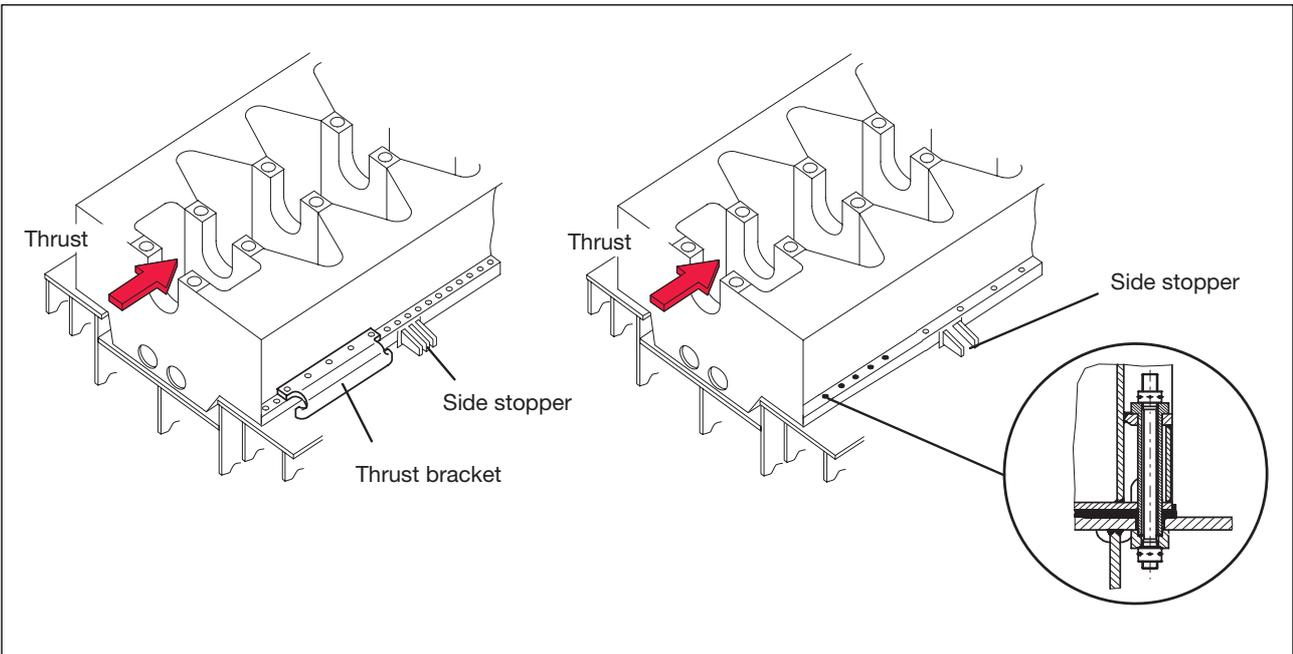
One important point which has been confirmed by shipyards, is the good access to all foundation bolts. The number of foundation bolts could be reduced by approximately 40 per cent compared with the RTA-U engines which also helps to save time during engine erection (Fig. 32). This advantage could also be retained in the RTA-8T Version B engines.
