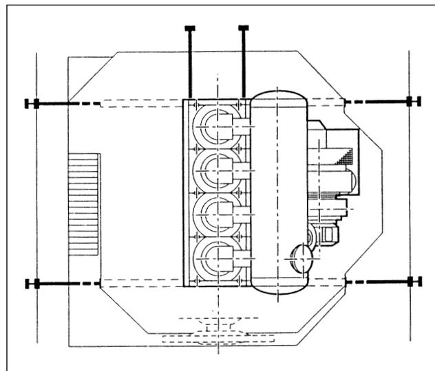
The usual remedy for lateral vibration amplitudes is to fit side stays at the engine top. These are normally required for engines with five and eight cylinders while provision for fitting them ought to be made with six-cylinder engines in case they are shown to be necessary during the sea trials (Fig. 41).
