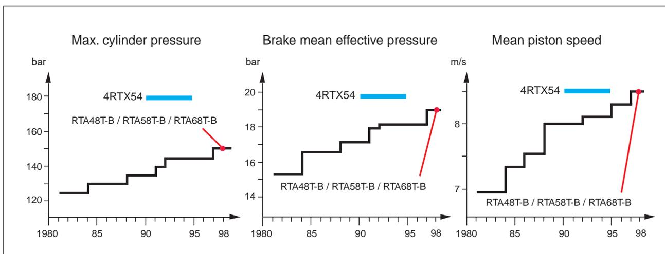
duced fuel consumption levels are possible at the previous power outputs. In certain cases, the increased output also helps to reduce the number of cylinders required.
