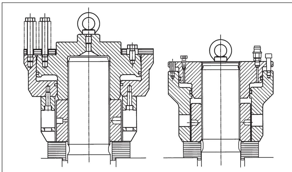
Fig. 12 Hydraulic jacks for the RTA58T (right) are much smaller than those for the RTA62U (left) [97#242]
