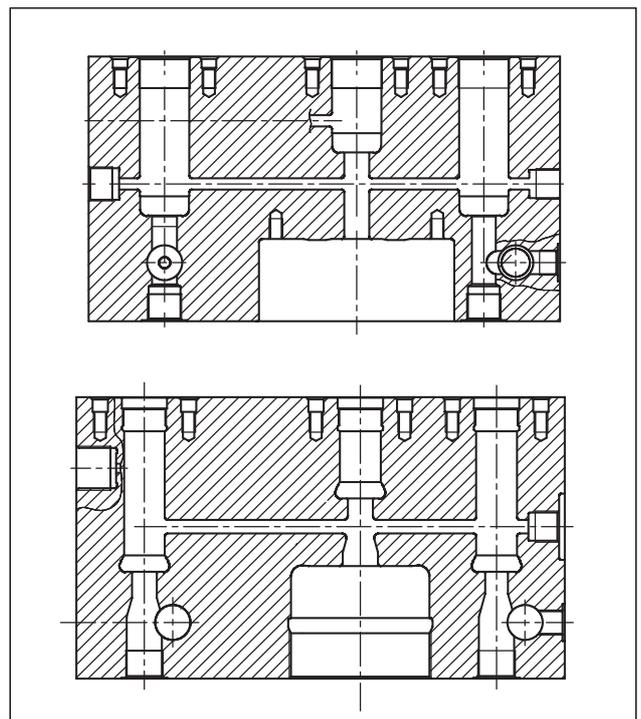
suction and spill valves, omission of recesses, same bore diameters wherever possible, etc. (Fig. 28). The new design has thereby significantly reduced the sensitivity of the housing to poor machining, and further increased the margin against cracks in the housing.
