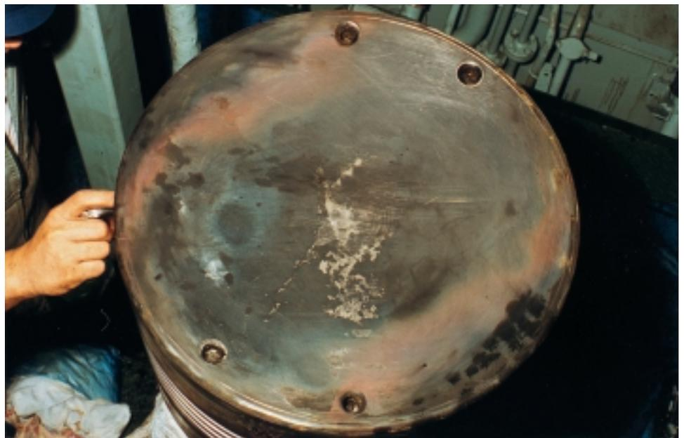
Additionally, the engine of *Star Sea Bird* was inspected after 2478 running hours and that of *Stena Commodore* after 1050 running hours. Basically the same information was collected as from the engine of the *Win Trader*. On *Star Sea Bird*, two pistons were pulled and one main bearing was inspected. The main bearing shell was found to be in satisfac-
