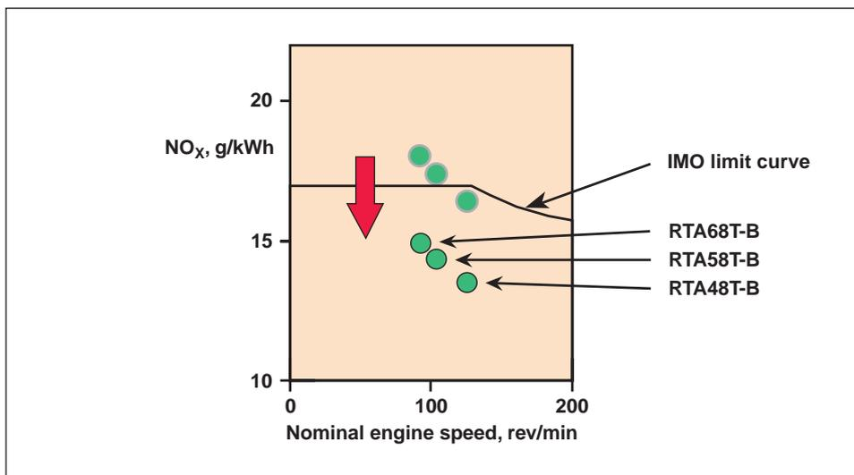
Fig. 11 Sulzer RTA-8T engines will comply with the prospective IMO regulations. As indicated here, the NO<sub>x</sub> emissions of RTA-8T Version B engines will be reduced to below the IMO limit by adaptation of tuning, particularly with the aid of the standard VIT system [98#107]
