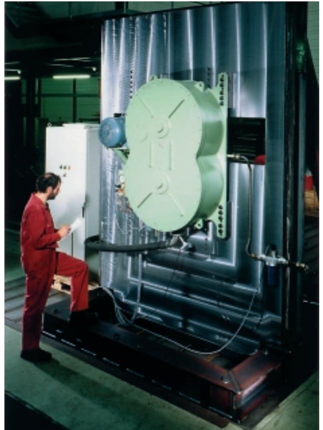
The first ELBA balancer was mounted on the 4RTA58T research engine in the Diesel Technology Center in Winterthur and was tested together with the engine (Fig. 42). Additionally, an endurance test of approximately 1000 hours has been carried out with the ELBA balancer on a test rig (Fig. 43). The first ELBA units have been ordered at H. Cegielski and Shanghai Shipyard, where the first engines equipped with ELBA balancers have now successfully passed their sea trials and are in service.
