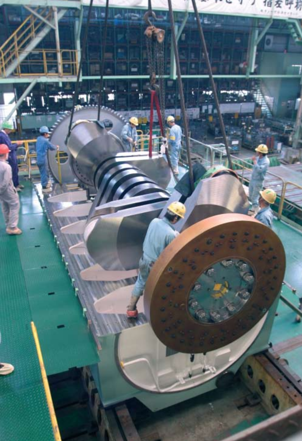
Lowering the crankshaft into the bedplate, 6RT-flex50.
