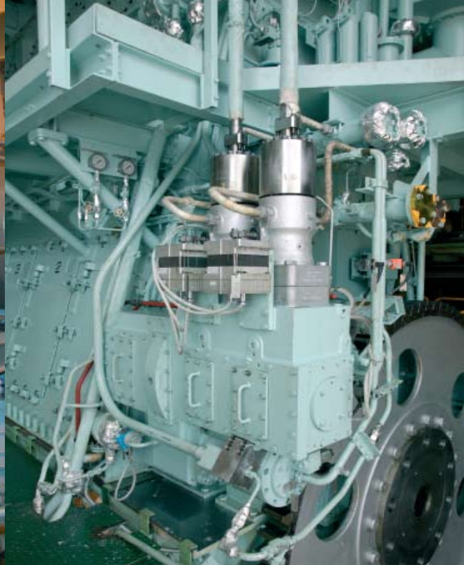
Supply unit of a 6RT-flex50 engine with fuel pumps vertically mounted on top and the servo pumps beneath and behind.
