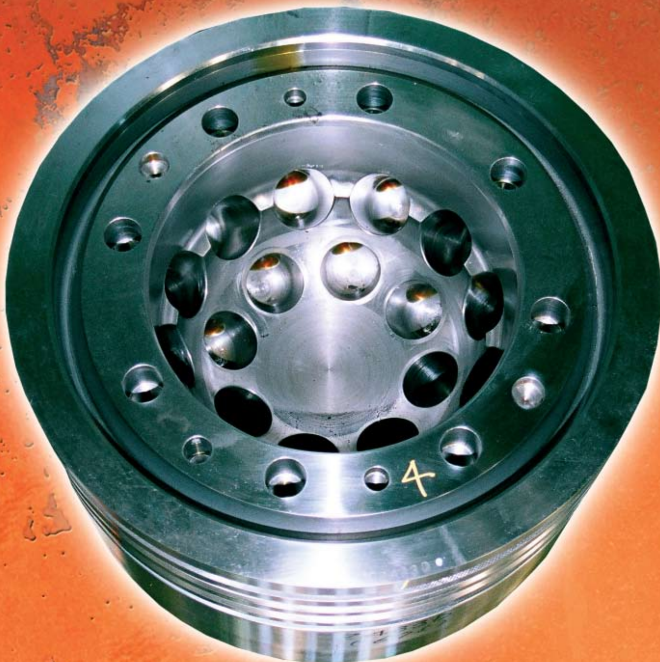
Piston underside showing the cooling bores.
