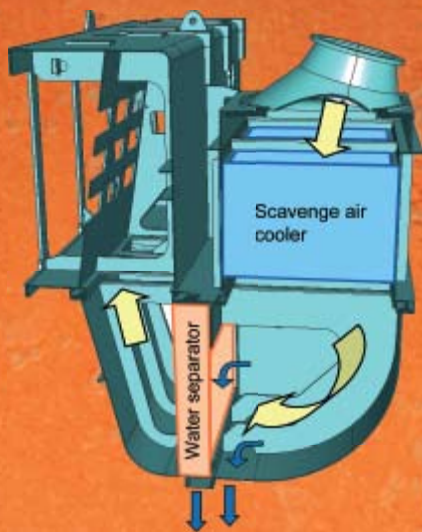
Scavenge air flow from the turbocharger through the horizontal scavenge air cooler and the vertically-mounted water separator, exiting left to the engine cylinders.
