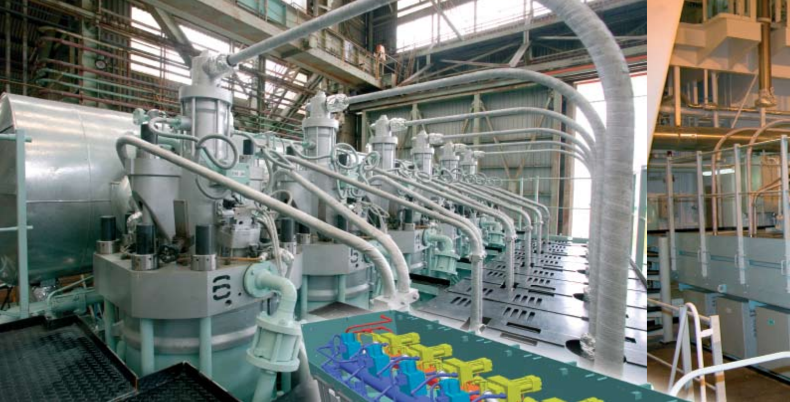
Cylinder top level of the RT-flex50 engine with the fuel injection and valve actuation pipes rising out of the rail unit under the platform.
