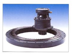
A Pel-Job exclusive: the radial piston slow slewing motor. This motor has a very high starting torque for flexible manoeuvres, and drives the crown directly without a mechanical reducer. The result is fewer moving parts and therefore less risk of wear. The automatic hydraulic brake incredintegrated in the slewing motor immobilises the turret in all positions and guarantees optimum working safety even on a slope.
