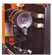
The radiators of the hydraulic circuit and engine are placed side by side to facilitate their cleaning. The battery and the air filter too are very easily accessible.
