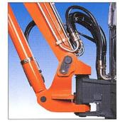
The sturdy boom king post provides a total range of movement of 130°. The double-fork pivot and the long king pin contribute to the assembly's rigidity. All the pins are fitted with bushes to ensure long life and to increase service intervals.
