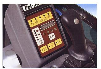
The PUMA system on the EB 706 continuously monitors all the machine's vital functions and immediately informs the operator if there is a fault. The operator is therefore free to concentrate fully on operating the machine.
