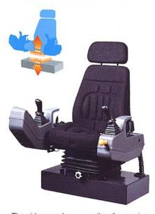
The side consoles supporting the manipulators are rigidly linked to the seat's suspension: operating precision is independent of the machine's movements and the operator is sure of finding an operating position ideally suited to him.
