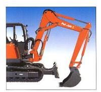
The new articulated boom increases the EB 706's versatility. The boom's additional joint reduces the equipment's overall dimensions and makes it possible to position the bucket on a larger ground surface, even in the immediate proximity of the machine.
