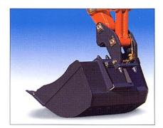
A Pel-Job exclusive: the quick coupling system enables bucket or accessory to be changed without the operator leaving the cab. Appreciated by all users, this device saves a lot of time and increases comfort considerably without altering the bucket's performances or sequence of operations.
