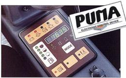
The PUMA system on the EB 30.4 continuously monitors all the machine's vital functions and immediately informs the operator if there is a fault. The operator is therefore free to concentrate fully on operating the machine.
