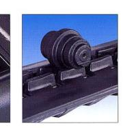
Ride comfort is considerably improved thanks to the profile of the tracks and the alternating position of the guides which provides permanent contact with the rollers
