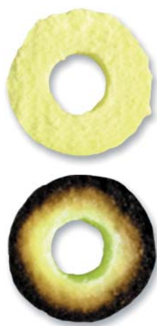
Cross section of absorption elements: New (above) and after 2.5 hour emulsion test according to IMO procedures (beyond).
