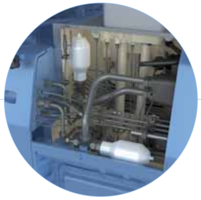
Pulsation dampers effectively reduce fuel pulses for improved safety.
