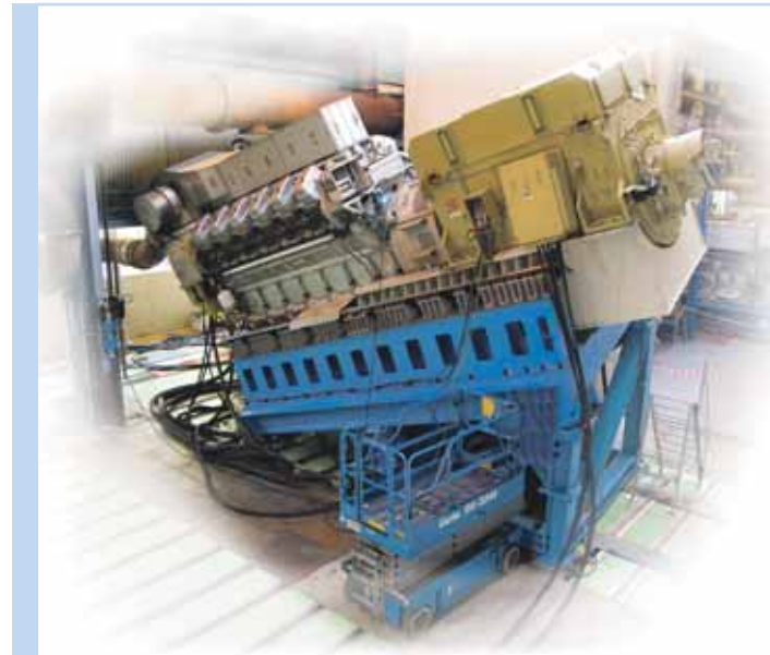
Bergen engines are type-approved for operation as emergency generator sets on mobile offshore drilling units after successful testing at 25 degrees of inclination.
