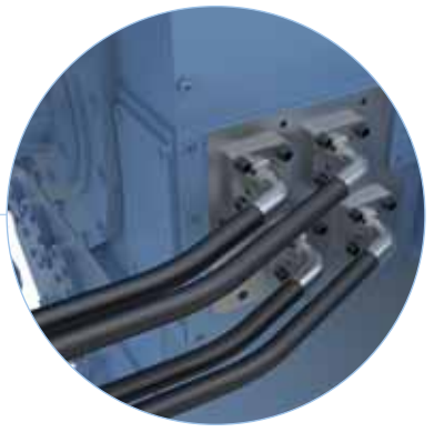
A pipe connection plate module carries all the fuel channels, for safe and easy installation and overhaul.
